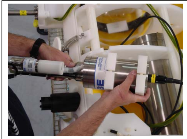
Figure 6: Lifting the CTD from the Sensor Mount
