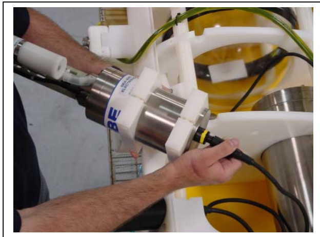
Figure 7: Unplugging the Bulkhead Connector
