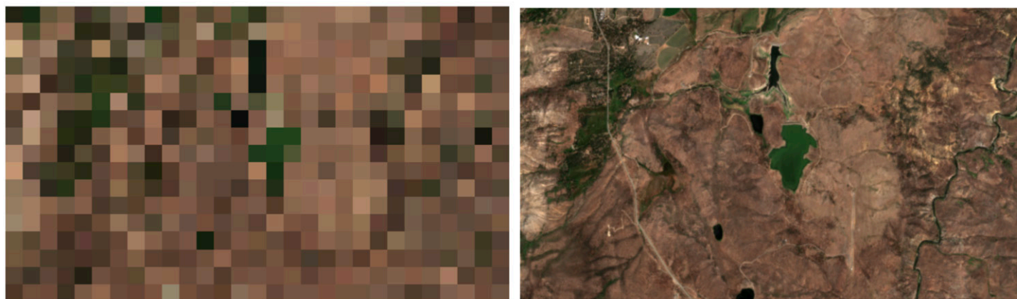
Fig. 1. A series of satellite images contrasting sensor resolution — medium-resolution (Sentinel-2, 10 m, Right) imagery that can resolve small lakes vs coarse (Sentinel-3, 300 m, Left) imagery that cannot.
