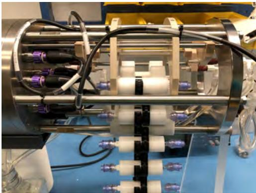
5. Continue to advance the cartridge chain (using **Load/Unload** mode) until there are an even amount of cartridges hanging below the RoCSI. This allows the chain to be completed by linking the first and last cartridges together.
