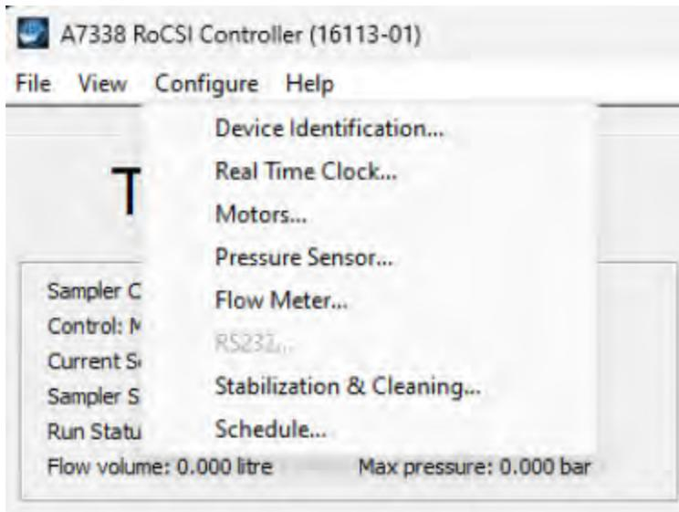
2. Select Sample Pump in the Motor drop-down menu. This allows direct control of the sample pump.
