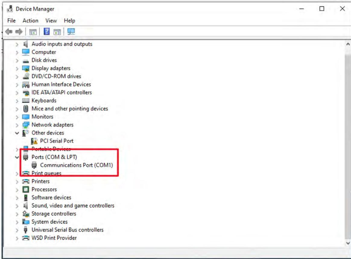
When plugging and unplugging the USB adapter to/from the computer, a port should appear and/or disappear from the Device Manager list of ports. This indicates the COM port that should be selected in benchmaps and that the device should communicate on.
