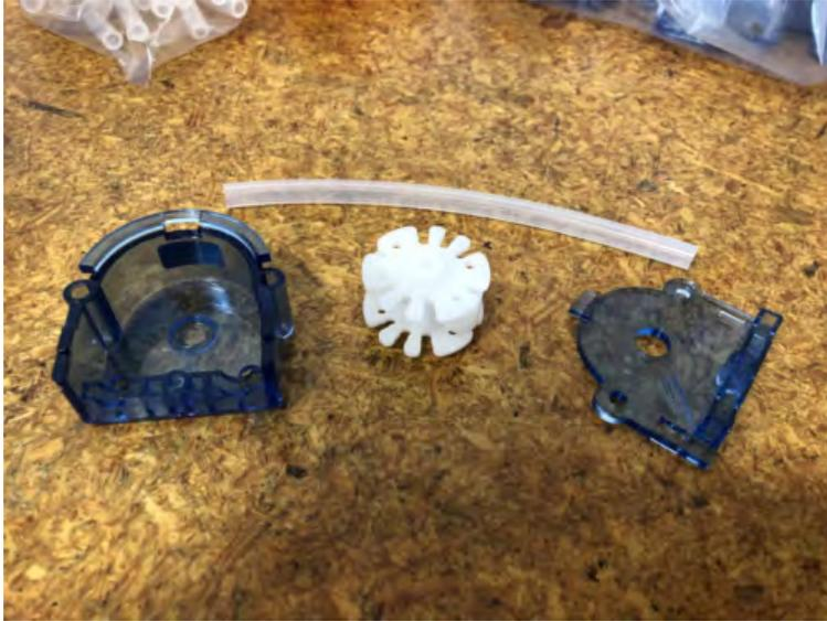
5. Remove the used tubing from the pump and disconnect any fittings that will be reused.
