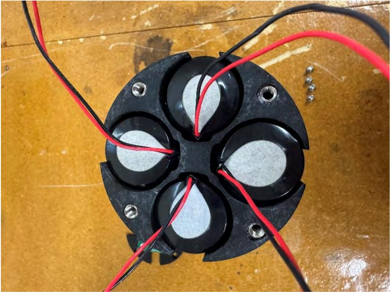
5. Take the 4 headers from the batteries and wrap them under the control board wrapping them clockwise. Two of the headers should line up with the J3 & J4 connectors of the control board.
