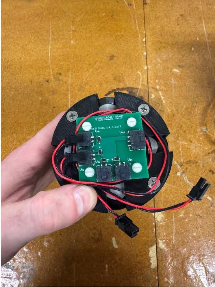
7. Insert the fully loaded battery pack into the housing. Ensure that the corner between J2 & J3 lines up with the sticker on the housing and end cap. This is to ensure the rubber bumpers on the end cap do not land directly on the connectors. Plug in the 3-pin header on the bulkhead to J5 on the control board. Align the end cap sticker ("1") with the housing sticker.
