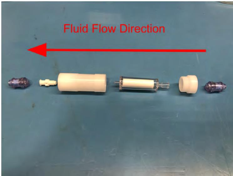
1. Noting the orientation of the parts shown above, start by screwing the Luer lock male to female connector into the sample holder using an 8 mm wrench.
