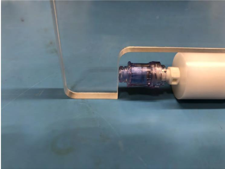
6. To begin creating a sample chain, install a chain link onto the cartridge as shown. Please note that in the orientation shown, water flow will be right to left.
