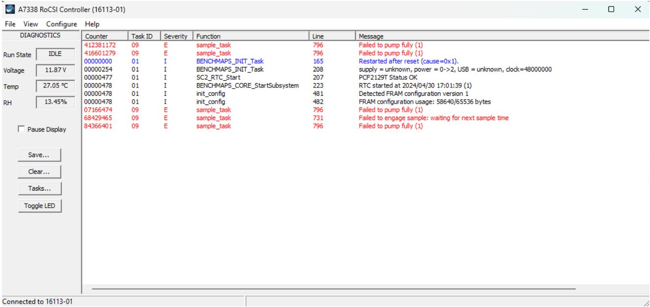
Clicking the **Tasks** button allows the user to configure the **DIAGNOSTICS** logging parameters. Messages may be turned on or off depending on the Log Filters (Error, Info and Debug). Typically, during regular operation only Errors are logged.
