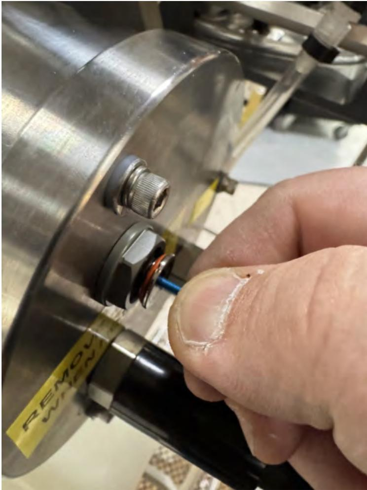
2. Loosen each end cap bolt a few turns at a time in a star pattern.
