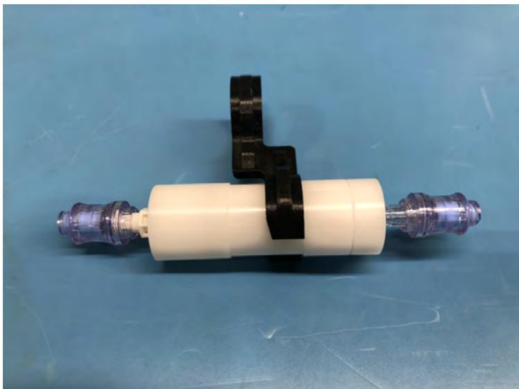
7. To begin creating a sample chain, install a chain link onto the cartridge as shown. The link is installed by firmly pushing it onto the reduced diameter section of the cartridge holder.
