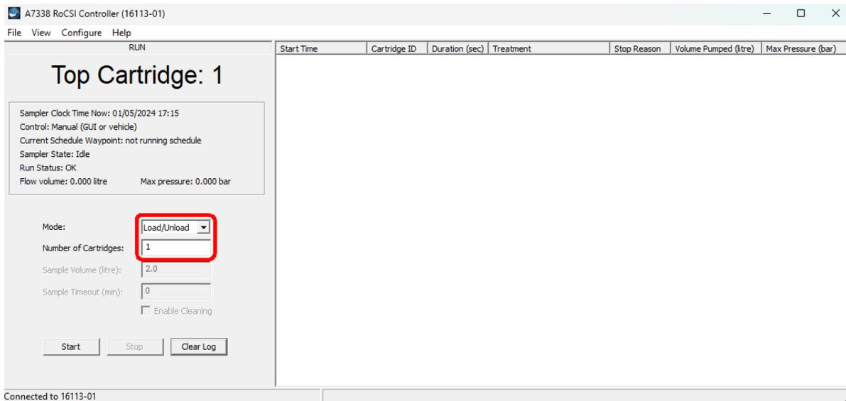
4. Gently hold the *first* cartridge (with no leading clip) against the loader wheel in the lowest accessible cartridge slot and click the **Start** button in the software. The cartridge should be pulled into position automatically.
