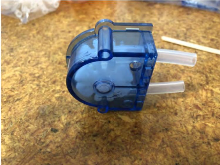
4. Separate the two halves of the pump housing. They are clipped together.
