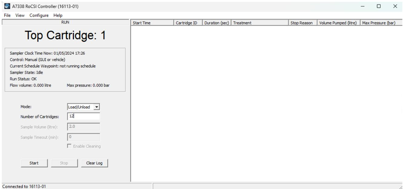
12. When the cycle is complete, the **Top Cartridge** is indicated as number 13. However, for this 12-sample chain, the top cartridge has returned to number 1. Reset the cartridge number by clicking on **Top Cartridge** and setting it back to 1.
