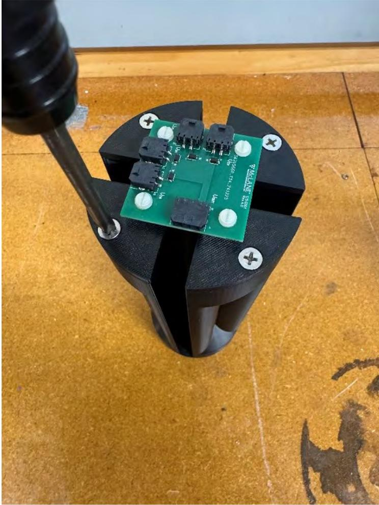
4. With the top plate removed, add the M4501 batteries to the battery pack. Ensure the wires of the battery are facing the center of the battery pack holder. This is to prevent the filled battery pack holder from getting stuck in the battery housing. Place the top plate back on the battery holder and screw the plate back onto the holder.
