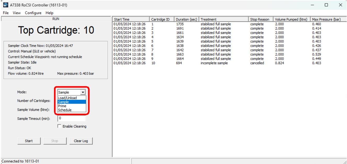
Loading and unloading, sampling, priming and scheduled sampling (modes) are initiated using the **Start** button. There is also a **Stop** button to terminate the current procedure and a **Clear Log** button to clear the sampler log and **Top Cartridge ID**.
