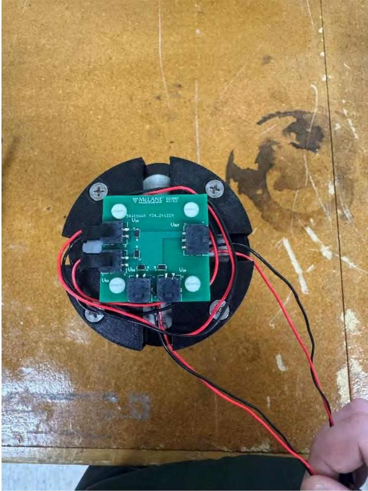
6. Wrap the remaining two headers counter clockwise and the two headers should line up with the J1 & J2 connectors on the control board.
