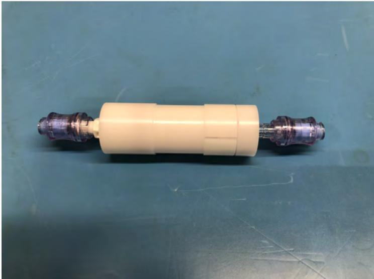
5. Use the gauge provided in the [toolkit](#) to ensure the cartridge is the correct length. The cartridge should gently slide into the gap and remain in position without falling out.
