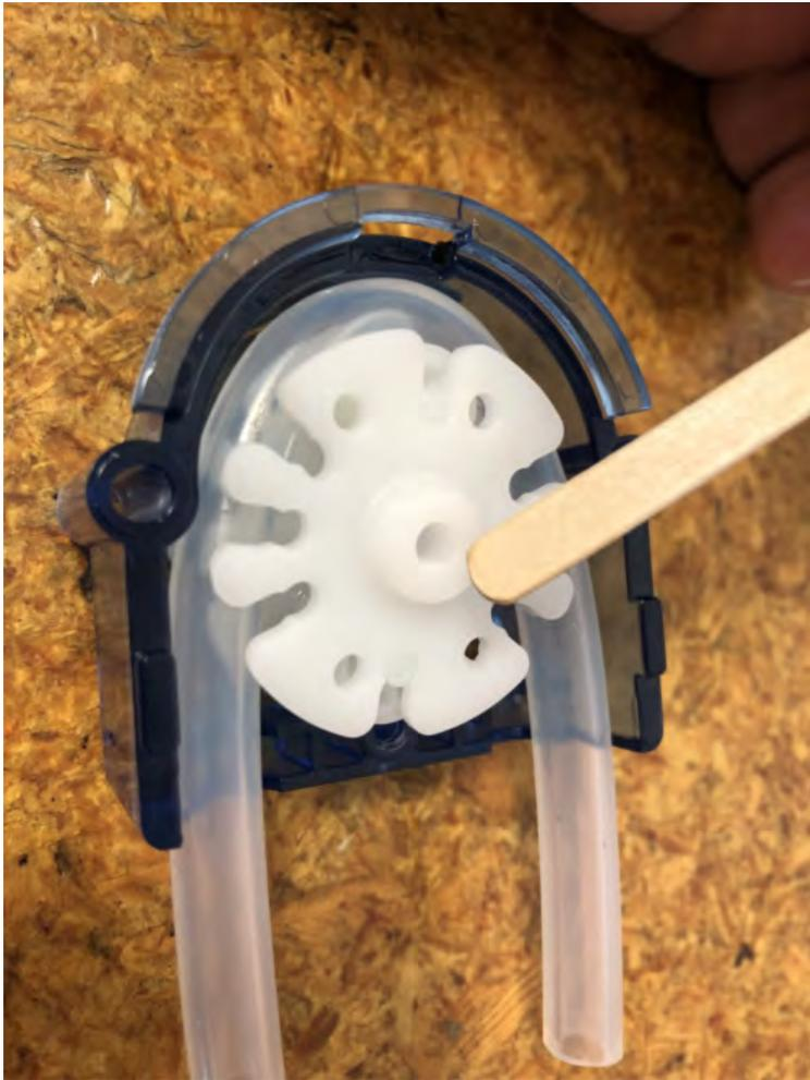
9. Replace the rear pump housing to secure the rotor and tubing in place.
