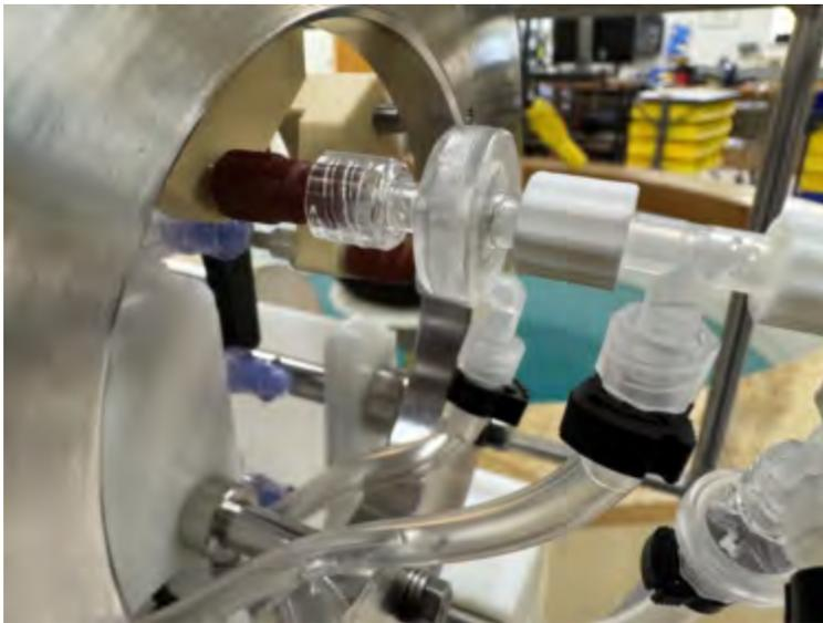
A second check valve is attached to the cleaner inlet, and will only need replacement occasionally.
