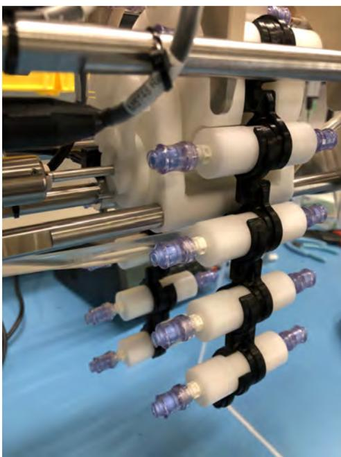
6. The magazine loader will be advanced until the sample chain is free of the mechanism. Please note that the weight of the chain must be supported while advancing the loading magazine. If not supported, there is a chance the drive mechanism may become jammed.
