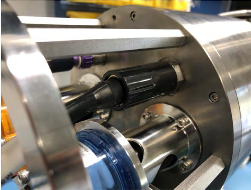
2. Next, plug in the USB connection to the host PC running windows. The computer should automatically find drivers in order to connect with RoCSI; this may take a few seconds to complete.
