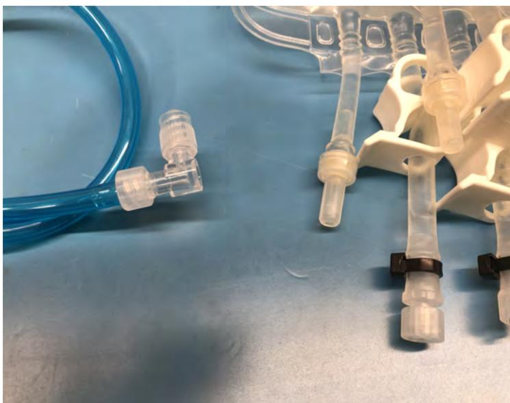
Fill each bag according to expected reagent use, and connect to the marked inlet tubes at each end of the instrument.
