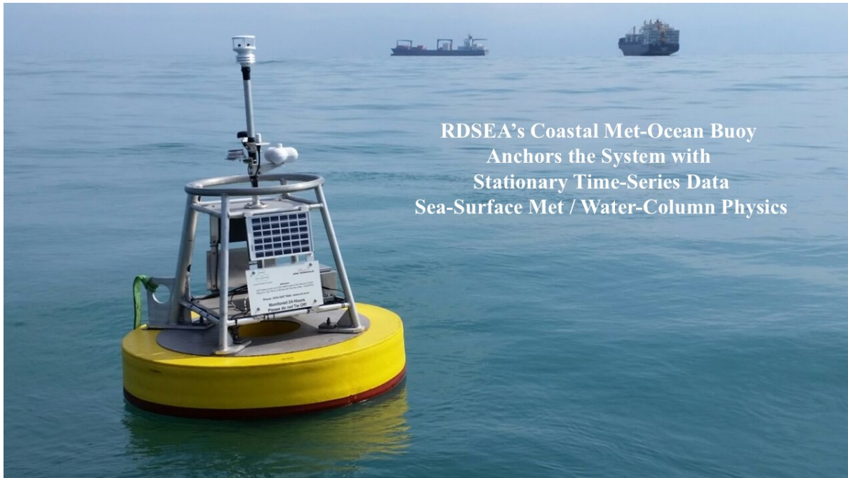
Figure 4: Deployed RDSEA MetOcean Hybrid Buoy System, used for stationary time-series monitoring
