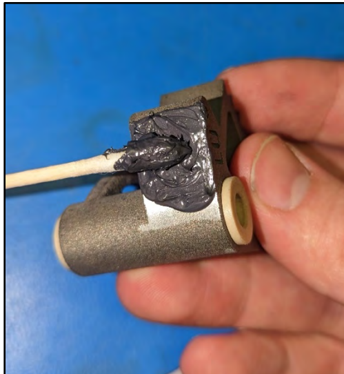
Figure 6-8: Apply thin coating of Bostik Black Moly anti-seize to each cam cleat
