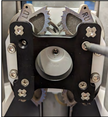
Figure 6-2: Remove cleat bridge
