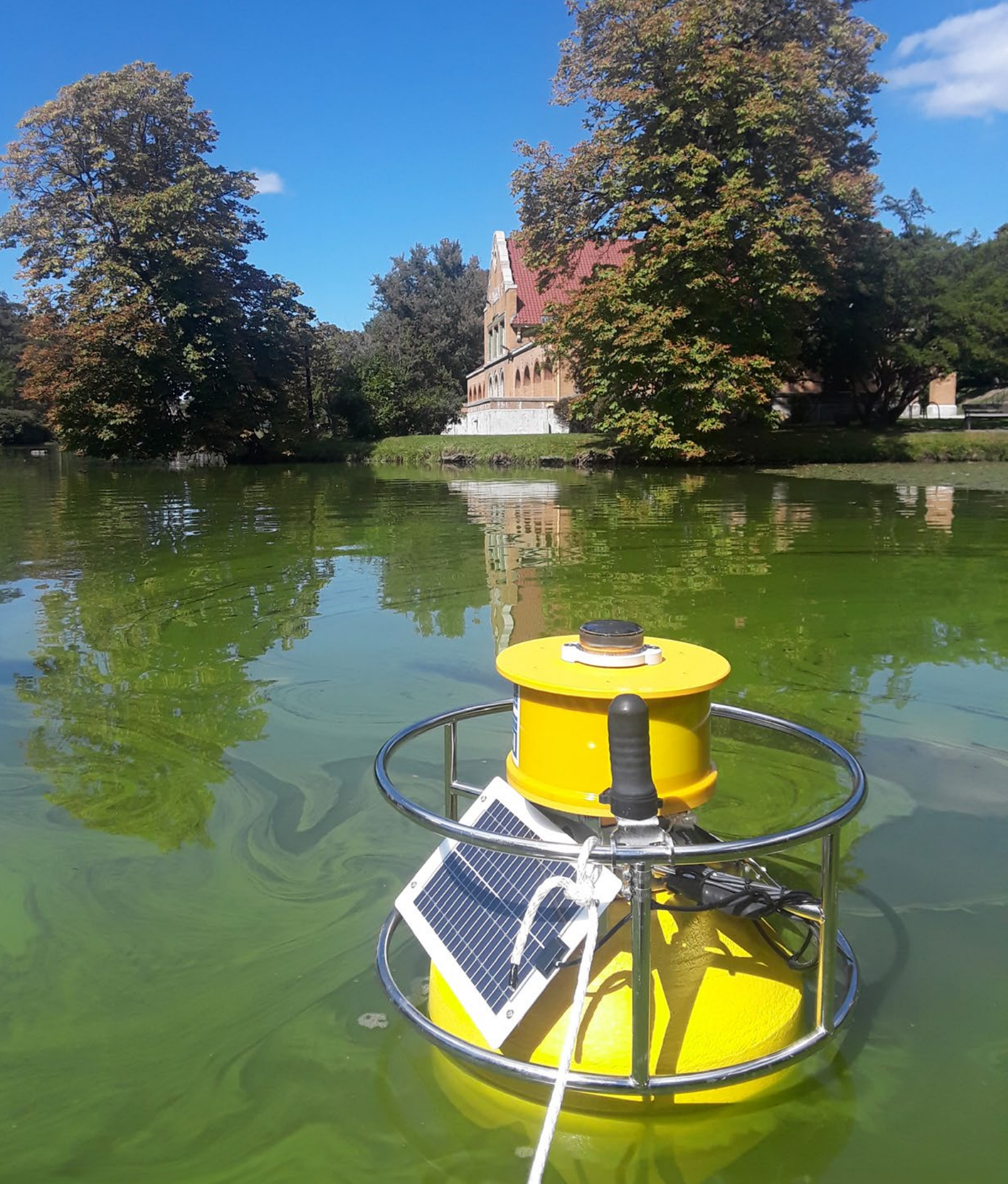
Water quality monitoring buoy deployed during algal bloom in Washington Park Lake, Albany, New York. Photo credit: M. Stouder.
