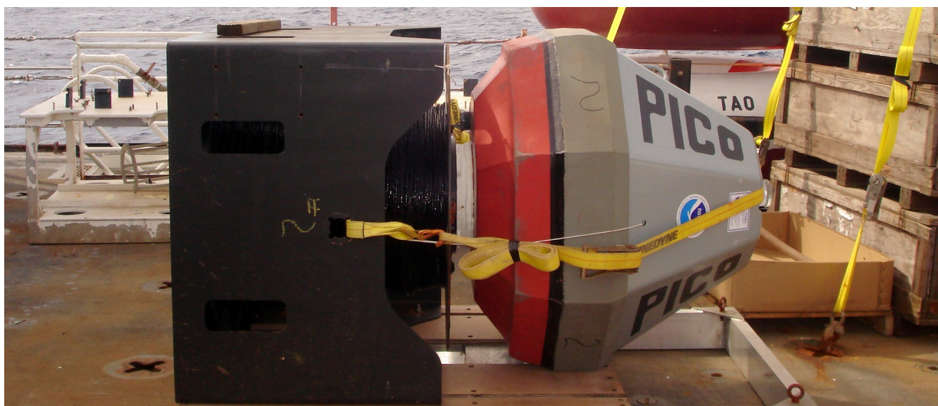
Fig. 1. The complete PICO mooring ready for deployment.
