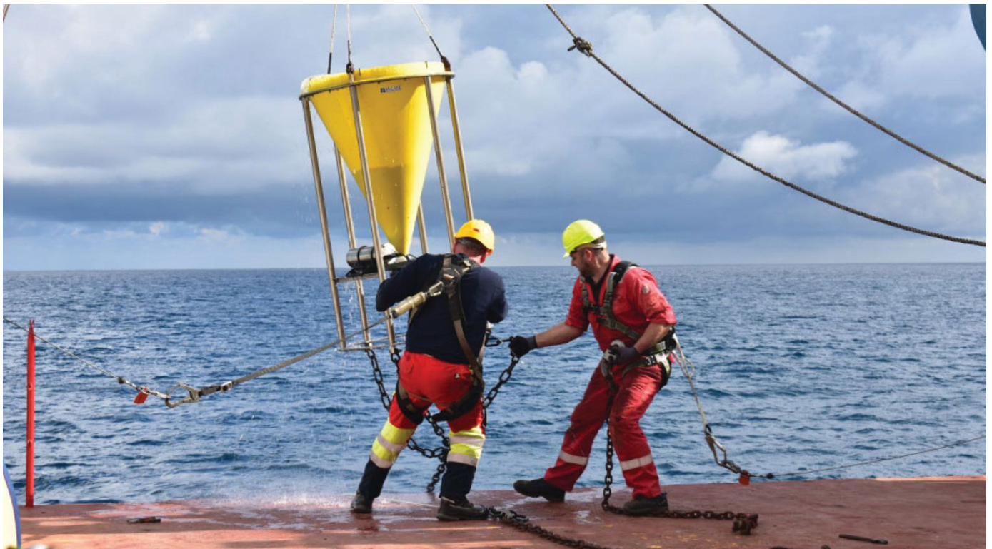
➤ Particle or sediment traps are funnel-shaped devices that capture sinking particles. (Credit: NOC)
