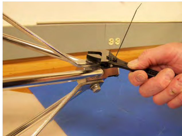
Figure A.3-8: Loosening Frame Guard
