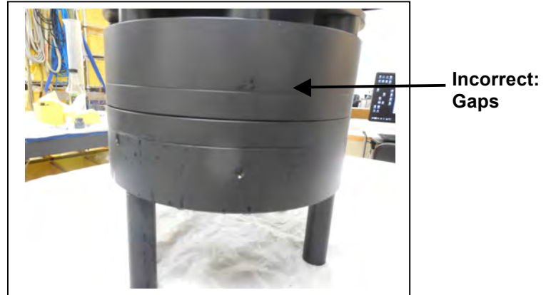
Figure 6-13: Incorrectly Closed Filter Holder
