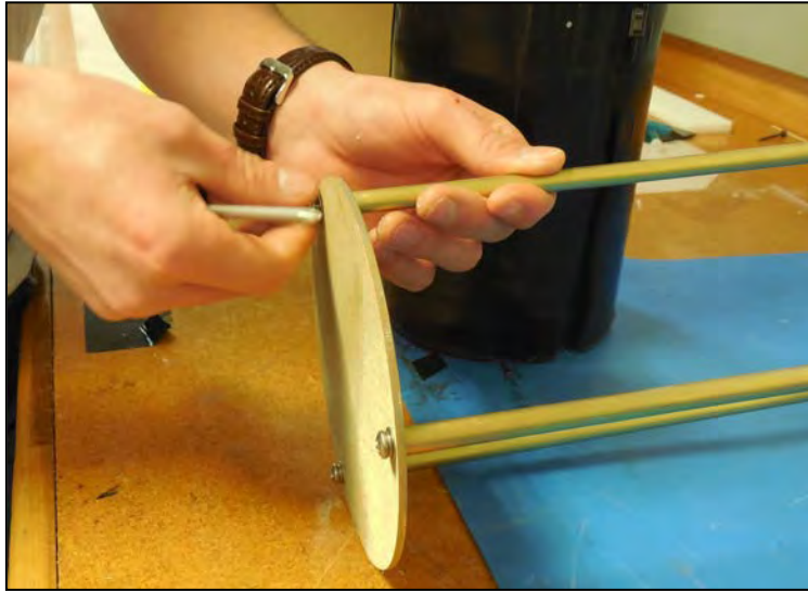
Figure A.2-3: Removing Battery Housing End Plate
