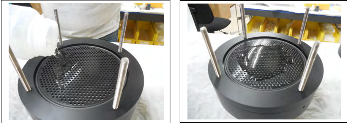
Figure 6-9: Fill the Pre-Filter Plate until Water Pools
