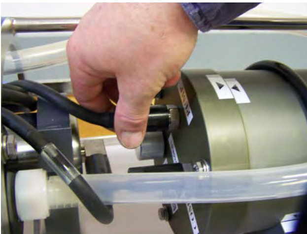
Figure A.3-7: Removing Connector
