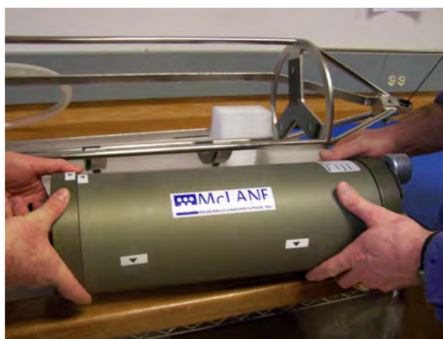
Figure A.3-12: Removing Controller Housing
