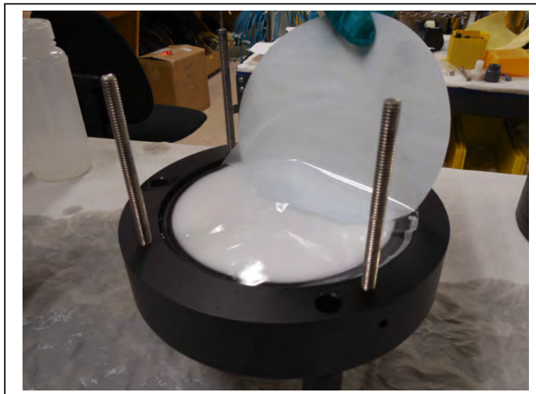
Figure 6-5: Placing the Filter on the Bottom Filter Holder Plate
