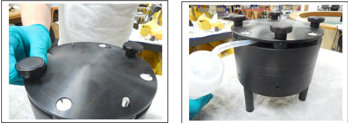
Figure 6-11: Tighten Nuts and Fill Assembly with Neutral Water
