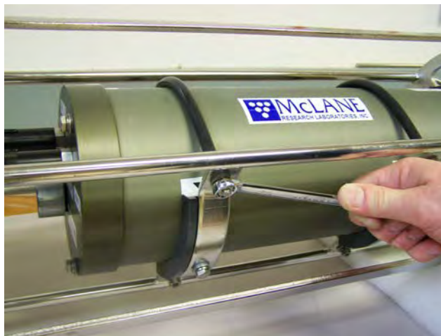
Figure A.3-10: Loosening U-Bolt Clamp
