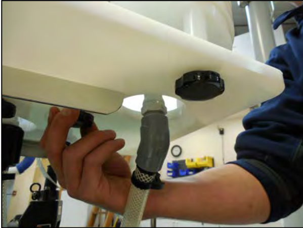
Figure A.1.2-3: Remove Nuts and Release Quick Disconnect
