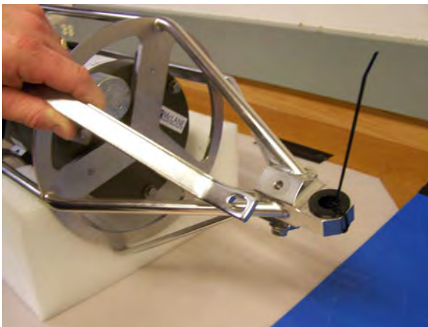
Figure A.3-9: Removing Leg Bolt
