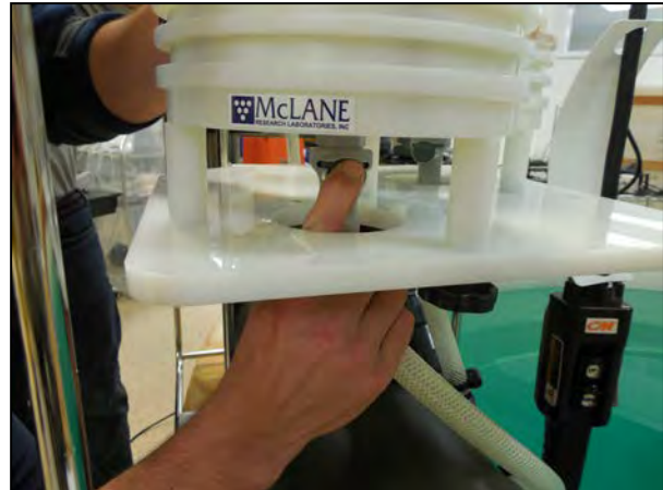
Figure A.1.2-3: Remove Nuts and Release Quick Disconnect
