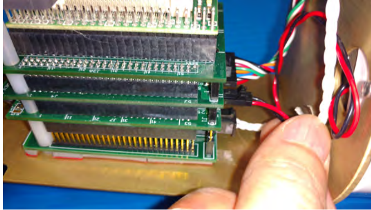
Figure 4-5: Connecting the Battery
