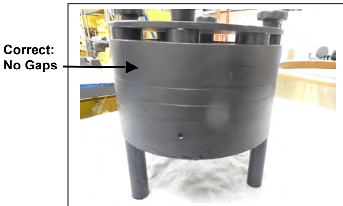
Figure 6-12: Correctly Closed Filter Holder
