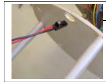
Figure A.1.3-6: Correctly Feeding Battery Connection Wires and Connecting Battery
