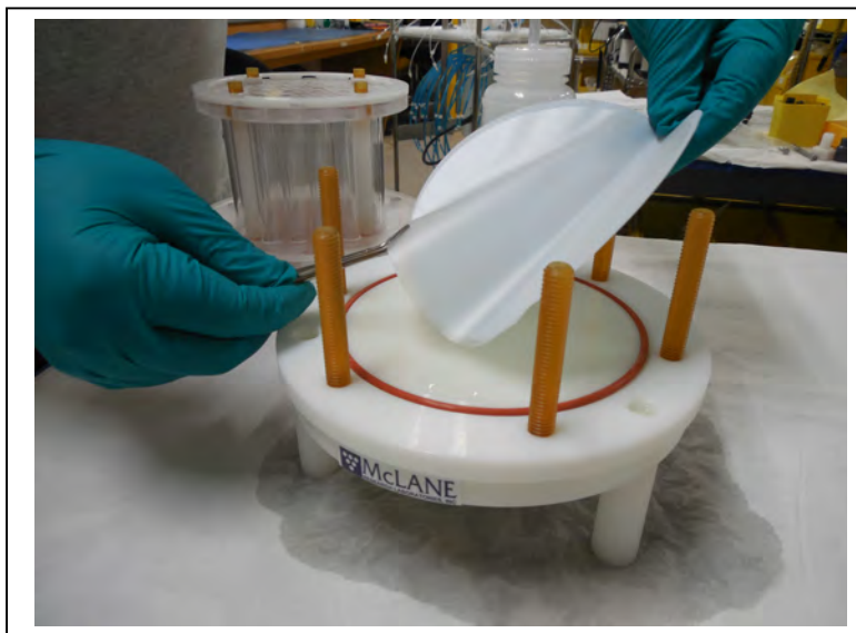
Figure 6-16: Placing the Filter onto the Filter Holder Plate
