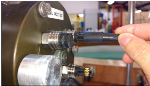
Figure 4-6: Connecting the COM Cable
