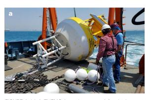
FIGURE 1. (a) A THEMO buoy is prepared for deployment in the eastern Mediterranean Sea off the coast of northern Israel. (b) The THEMO Shallow Buoy is a 2.25 m discuss buoy equipped for near-real-time reporting of MetOcean parameters and with downward-looking ADCP.
