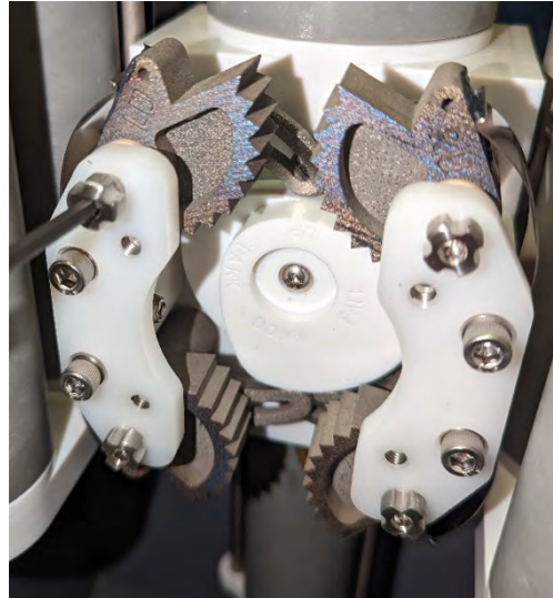
Figure 6-9: Fully tighten cleats
