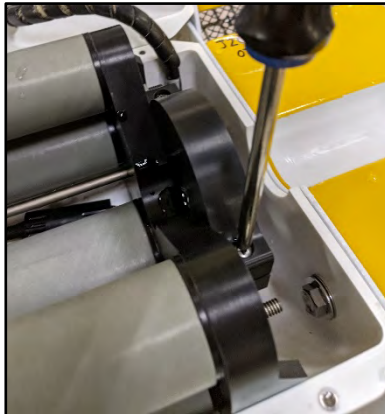
Figure 4-3: Remove screws on inductive floater
