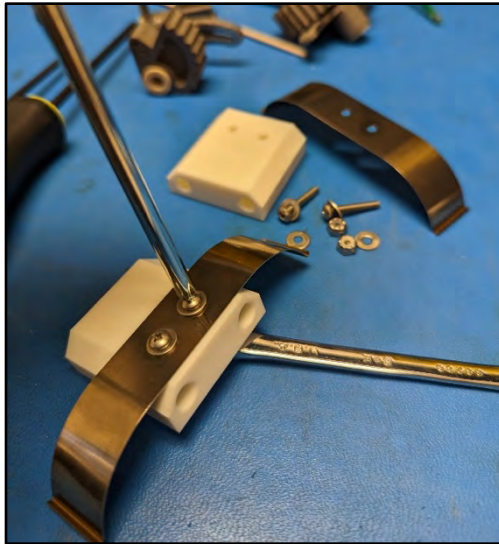
Figure 6-5: Remove springs from side plate
