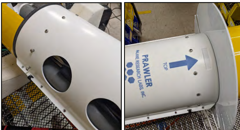
Figure 2-9: Re-attach core assembly to outer shell
