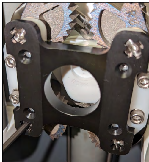
Figure 6-10: Attach bridge plate to assembly
