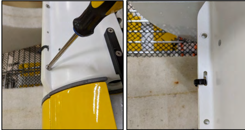
Figure 4-2: Remove screws on Prawler outer edge
