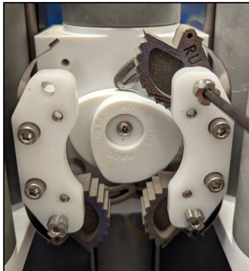
Figure 6-3: Remove cam cleat screws
