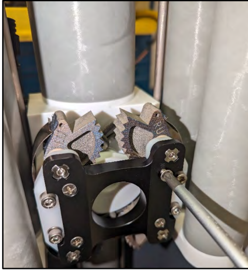
Figure 6-11: Fully tighten side plate screws
