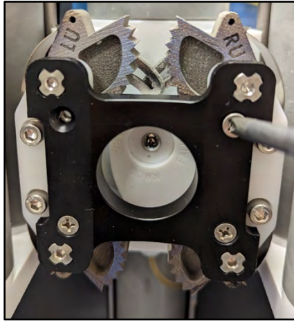
Figure 6-2: Remove cleat bridge
