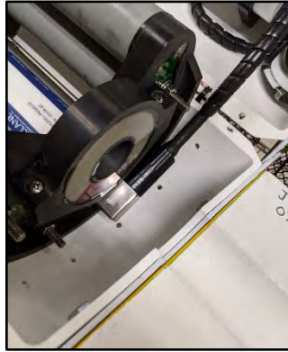
Figure 2-4: Disconnect CTD cable
