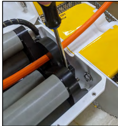
Figure 4-5: Attach inductive floater
