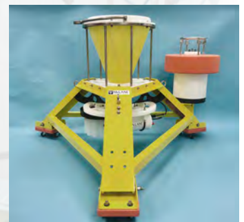
Top: Standard Sediment Trap & 8-13 Small Cone Sediment Trap Bottom: SABL Sediment Trap
