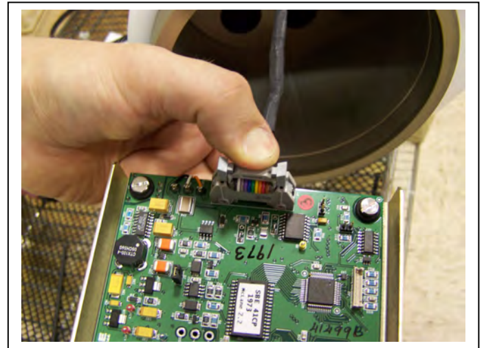
Figure 4-23: Connect CTD Cable
