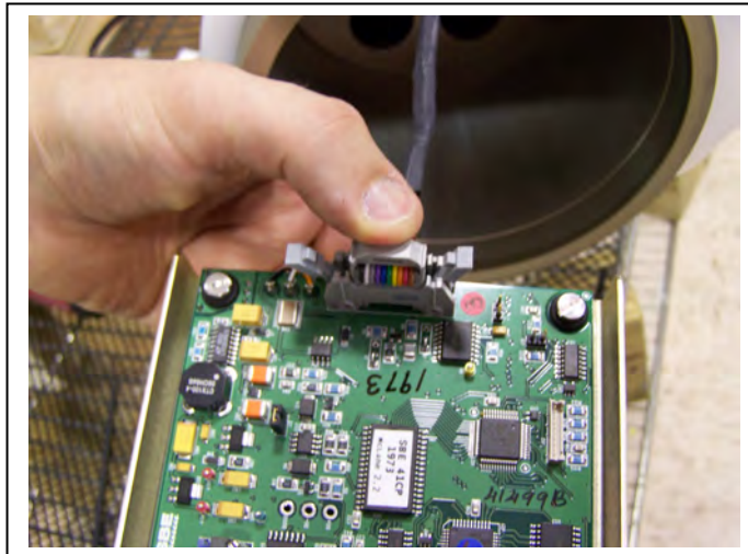
Figure 4-23: Connect CTD Cable
