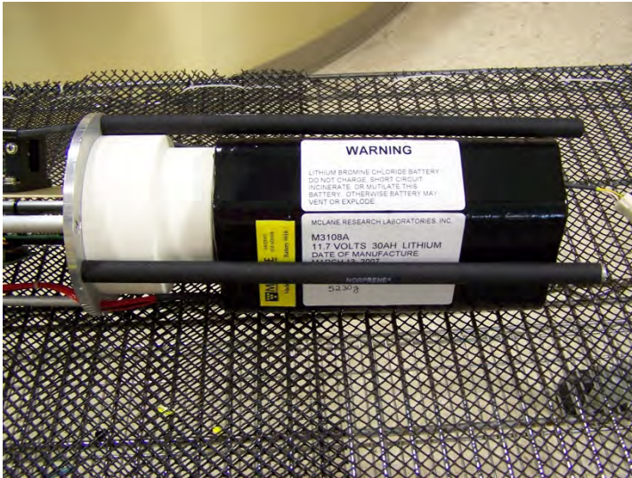
Figure 4-10: Battery Installed in Battery Holder
