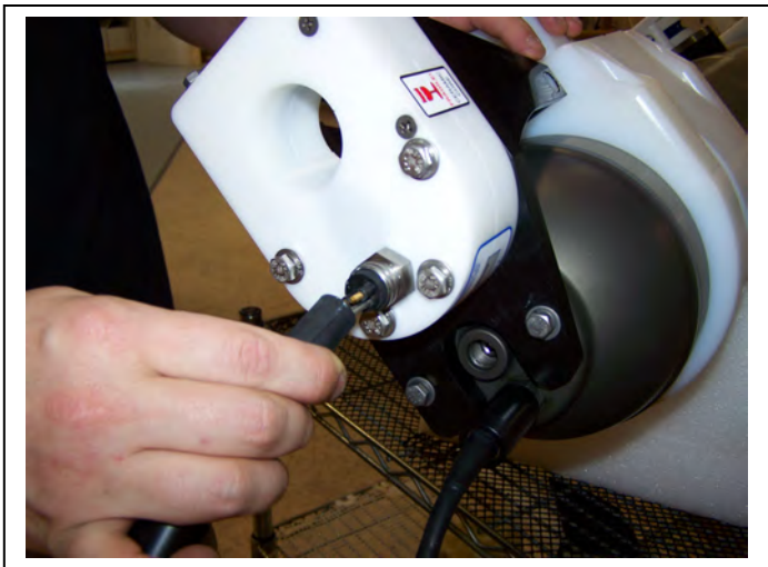
Figure 4-34: Connect UIM Cable
