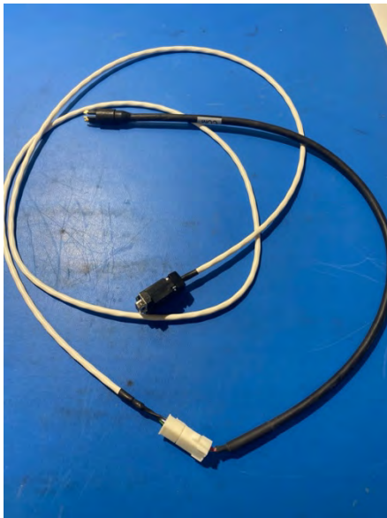
Figure 4-8: Communications Cable and USB to RS-232 Adapter
