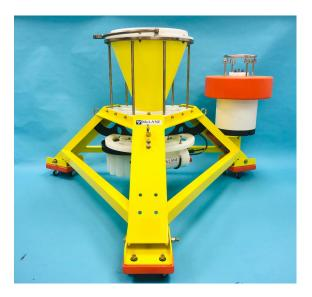
McLane's **NEW** Signal Activated Bottom Lander (SABL) Sediment Trap World Premiere will be at **Ol22 in Stand A525.** SABL targets specific discharge or re-suspension events. Features include:
