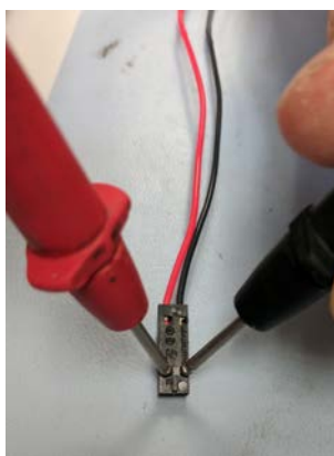
Figure 2: Measuring Battery Connector Voltage
