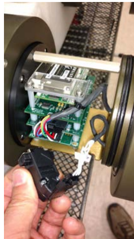
Figure 7: Plug MTE Connector into Loopback Tester
