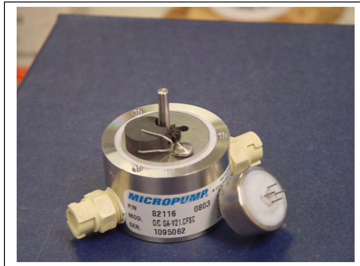
Figure 4-6: Pump Head Gear and Replaceable Magnet
