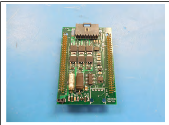
Figure 5-3: Three Phase Board
