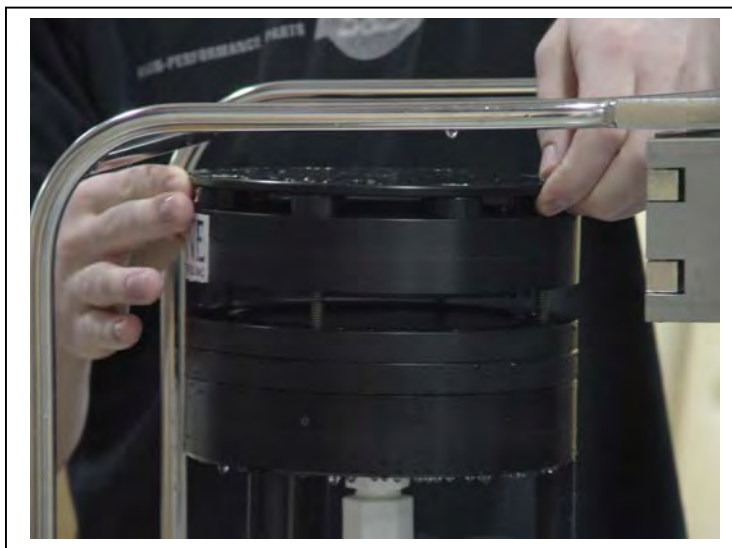
Figure B-2: WTS-LV 3-Tier Filter Holder
