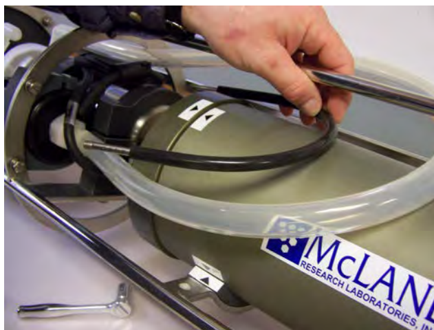
Figure A.3-11: Removing U-Bolt
