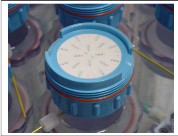
Figure 6-5: Sample Tube with Filter Holder
