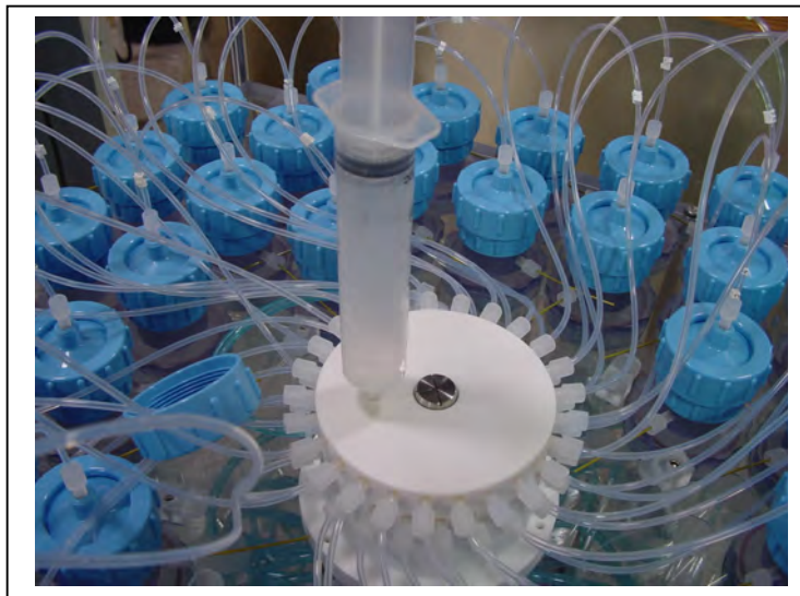
Figure 6-12: Injecting Water into the Valve Intake
