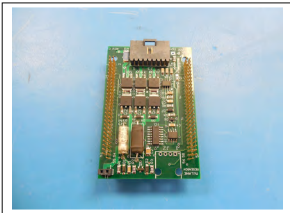
Figure 5-3: Three Phase Board
