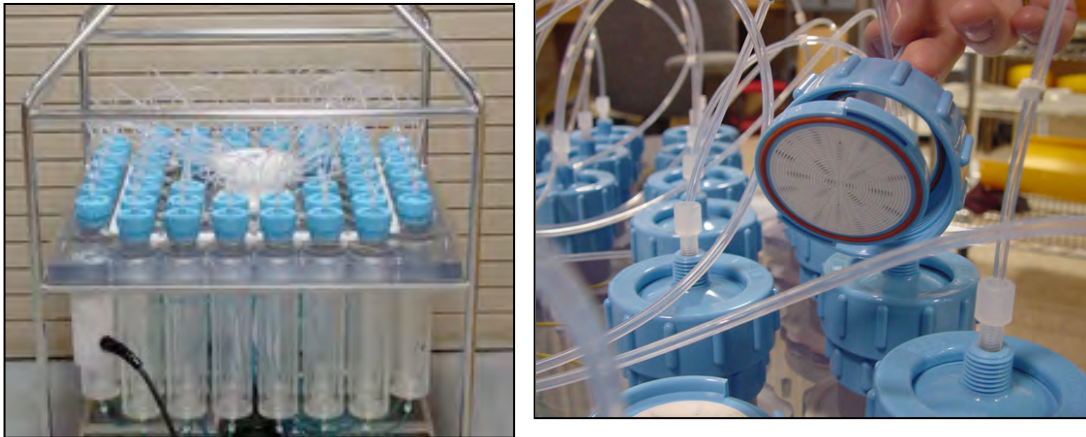
Figure 4-5: RAS-500 with Optional Filter Holder on each Sample
