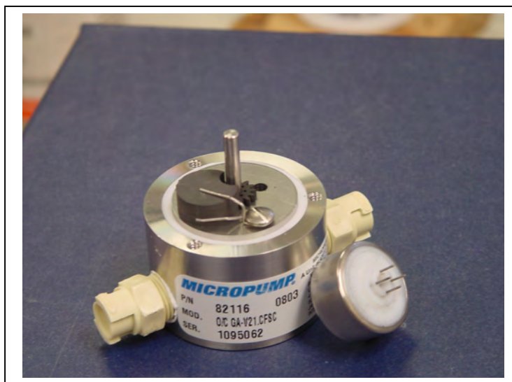
Figure 4-6: Pump Head Gear and Replaceable Magnet
