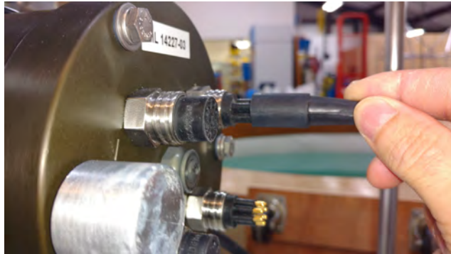
Figure 2-8: Connecting the COM Cable
