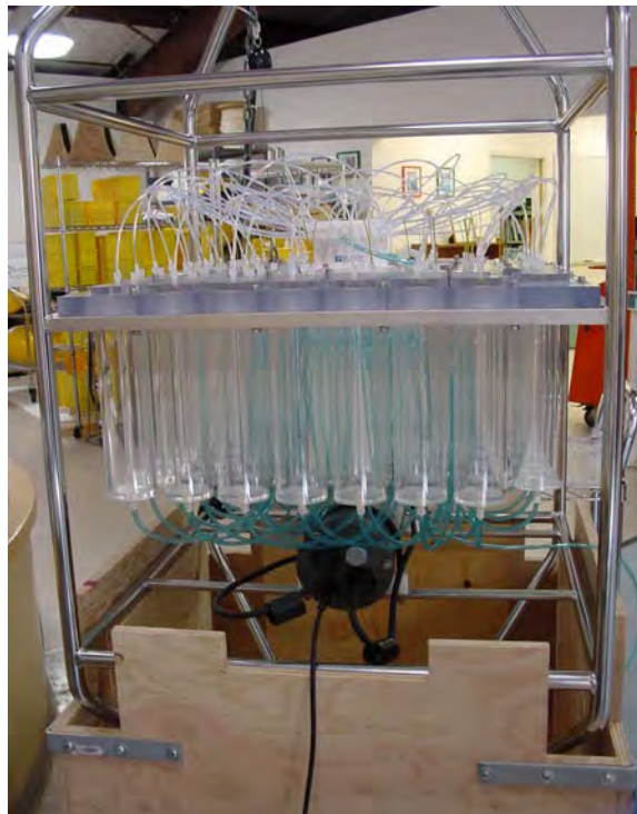
Figure C-3: Remove Controller Housing through Notch in Stand
