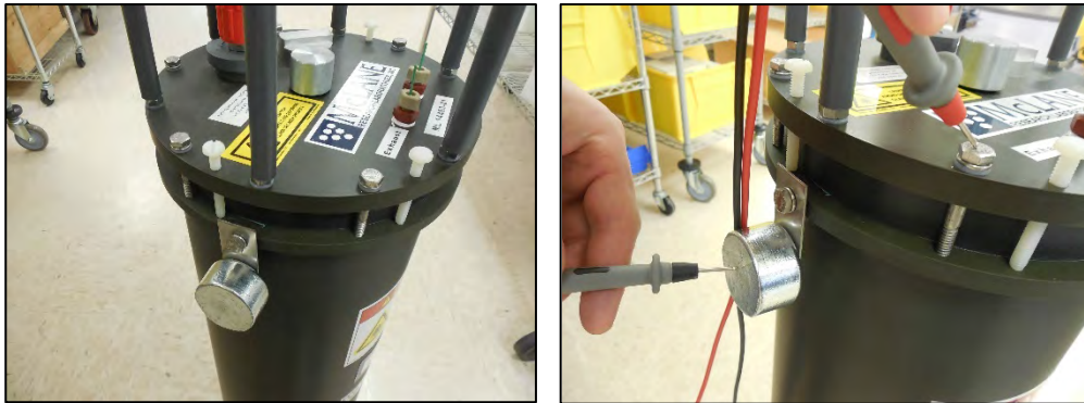
Figure 7-2: Measuring Tab Anodes of Bolt Rings and End Cap Bolts
