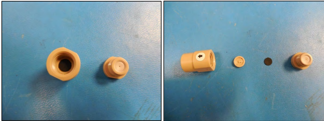
Figure E-64: Remove all Check Valve Parts
