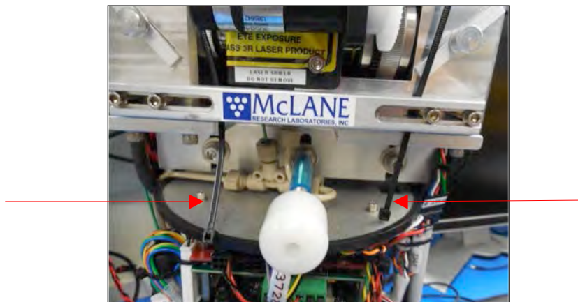
Figure 6.3.2-4: Insert Plastic Tie-Wraps on Alignment Bar
