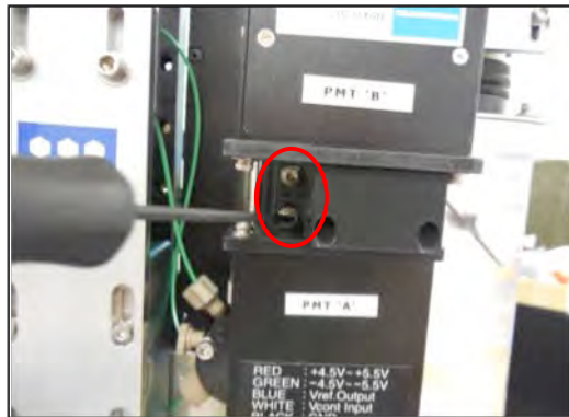
Figure A-31: Adjust PMT Mount Assembly Height
