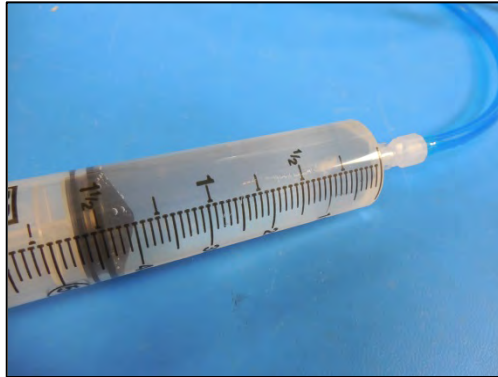
Figure 6.1-5: Fill Syringe and Connect to Fill Tube
