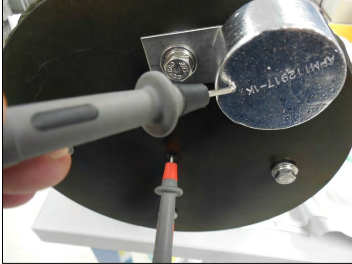
Figure 7-3: Measuring Housing Bottom Anode Resistance
