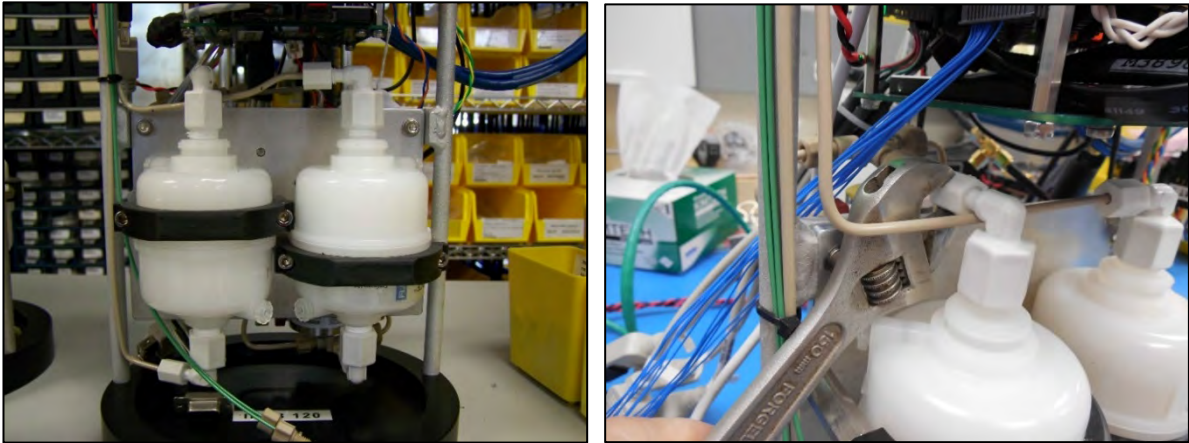
Figure E-70: Loosen White Hex Nut Fluidic Connections
