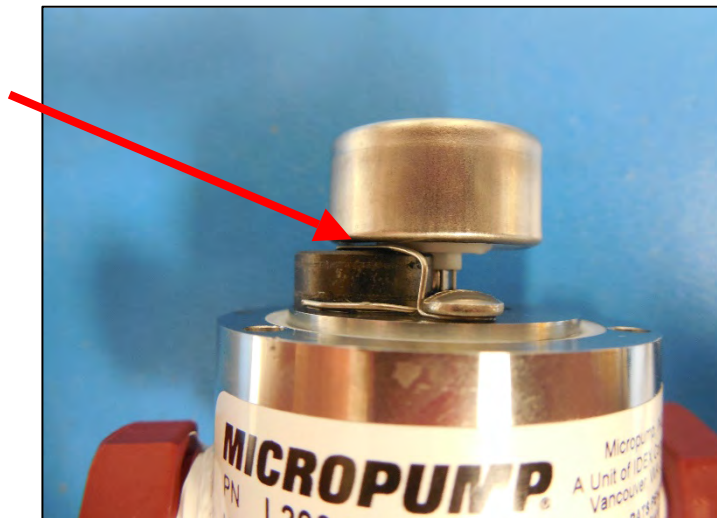
Figure E-32: Confirm Visible Gap
