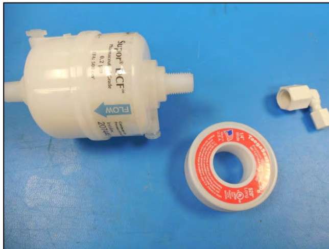
Figure E-73: Remove White Elbow Fittings from Existing Cartridge
