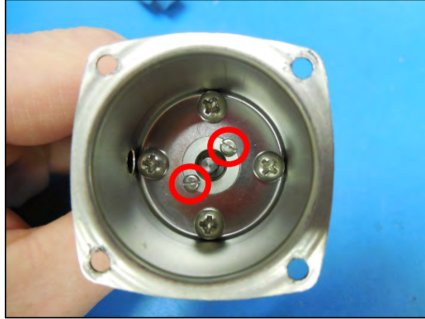
Figure E-23: Secure Motor with Screws
