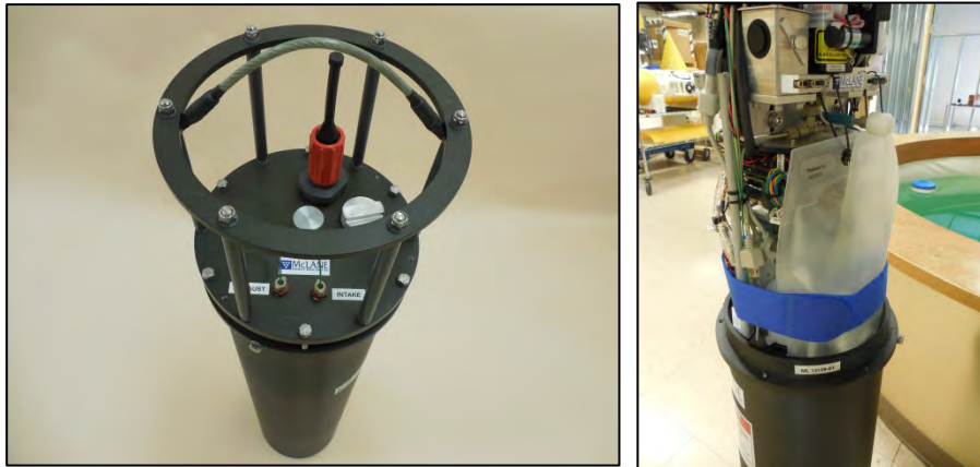
Figure 6.1-1: Remove IFCB from Housing
