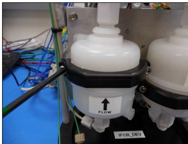
Figure E-77: Secure Clamp with Screws
