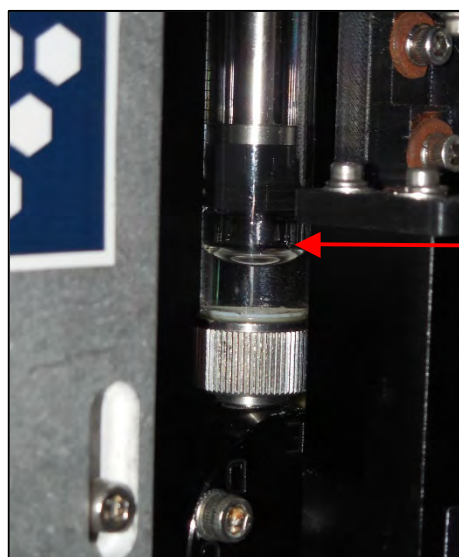
Example: needs further priming, excess gas in syringe
