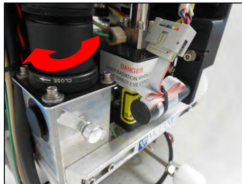
Figure A-19: Rotate Iris Ring
