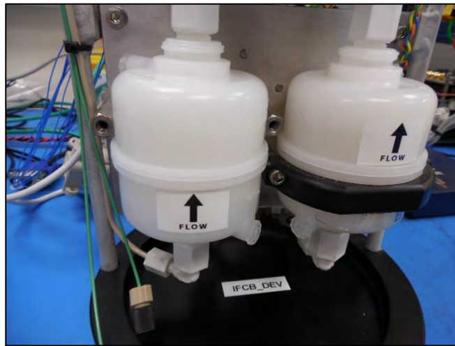
Figure E-76: Secure Filter in Place with Black Clamp
