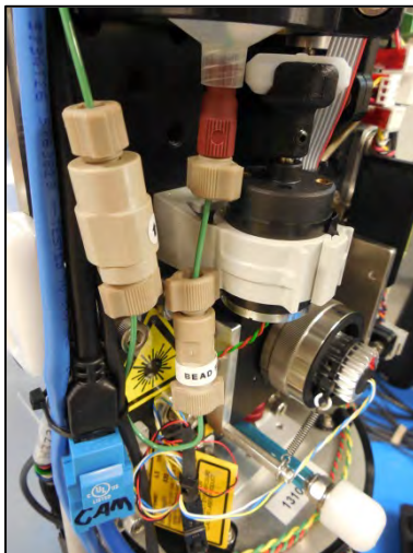
Figure 6.3.3-1: Assembly and Bead Fill Port
