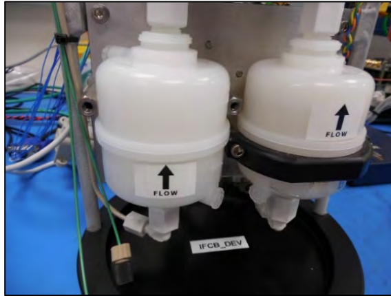
Figure E-72: To Reuse Fill Port O-Rings, Remove Each O-Ring
