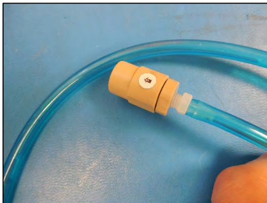
Figure E-68: Connect Check Valve to Opposite End of Valve
