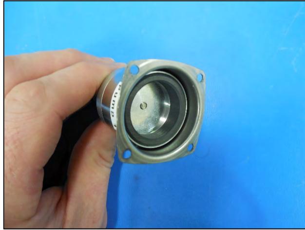
Figure E-25: Check that Drive Magnet Spins Freely
