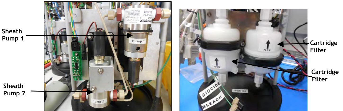
Figure 4-5: Sheath Pump 1 and 2
