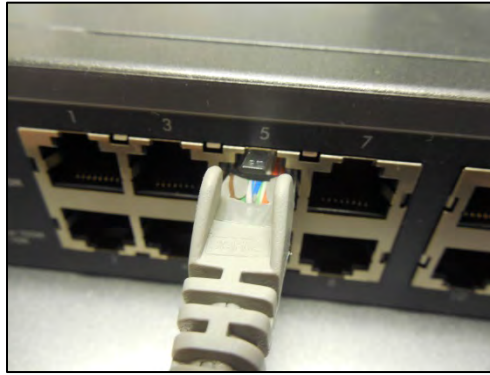
Figure 6.1-14: Connect Ethernet to Local Network
