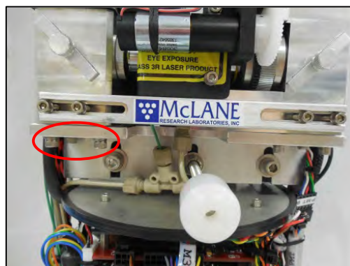
Figure A-17: Loosen Screws that Secure Condenser
