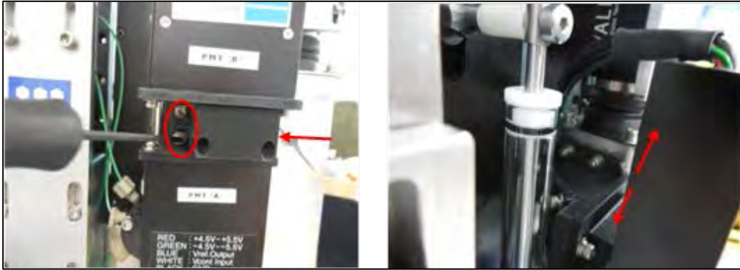
Figure B-2: Loosen Flange Screws, Slide Splitter Assembly Up or Down
