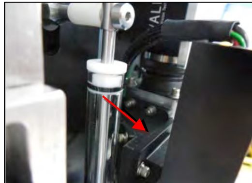
Figure A-31: Adjust PMT Mount Assembly Height
