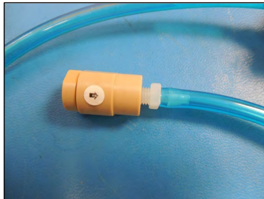
Figure E-62: Connect Bead Syringe to Opposite Check Valve End
