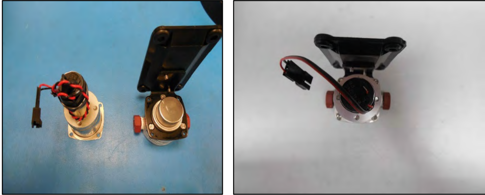
Figure E-35: Reattach Motor to Pump Head
