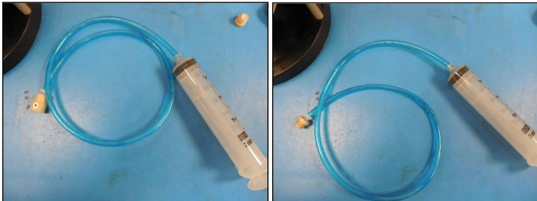
Figure E-65: Force Water Through Each Fitting
