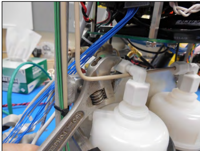
Figure E-78: Push Tubing Back into White Fluidic Connections
