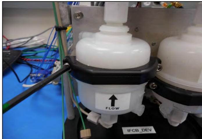
Figure E-71: Loosen Screws on Black Saddle Clamp
