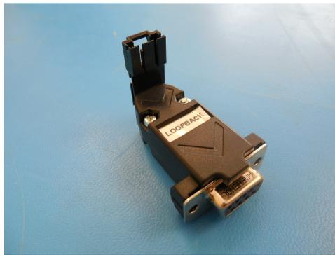
*Figure 4: Loopback Tester*
