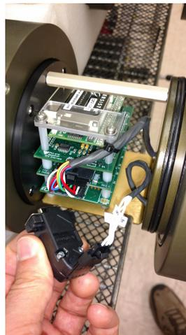
*Figure 7: Plug MTE Connector into Loopback Tester*
