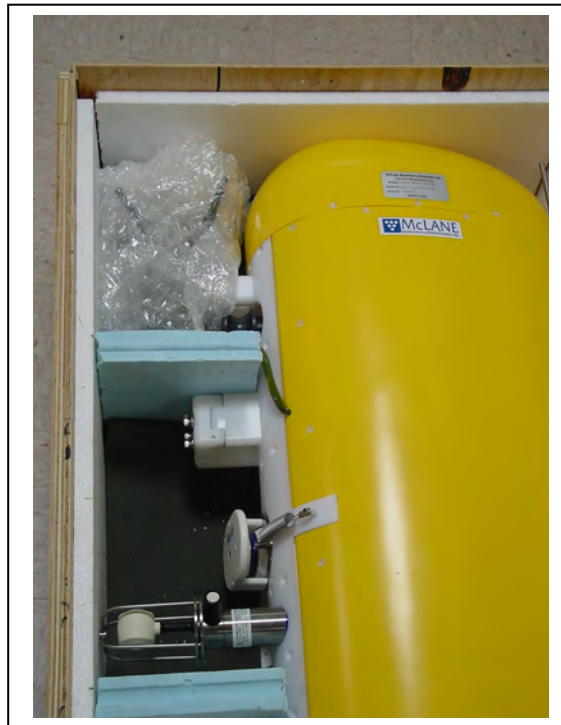
Figure 7-10: Fitting the MMP in the Crate
