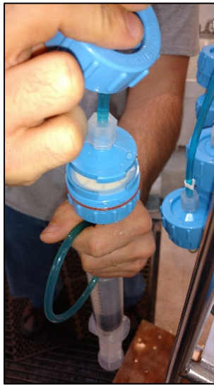
Figure 6-4: Reattaching Top and Bottom of Filter
