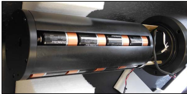
Figure 2-12: Drop-in Battery Holder for 'D' Cell Batteries
