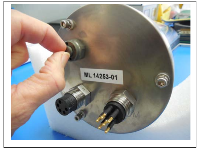
Figure 4-2: Releasing Pressure Relief Valve (Flat Style)
