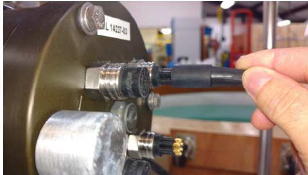
Figure 4-6: Connecting the COM Cable
