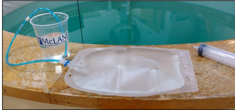
Figure 6-8: Place Hose-F into Fixative Container
