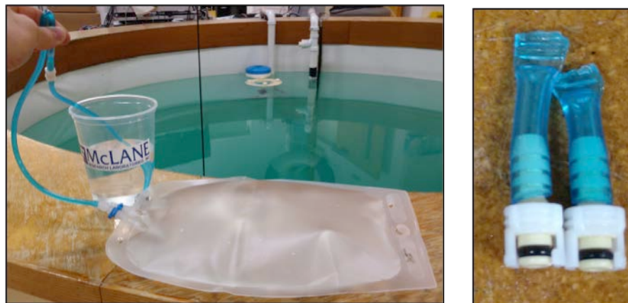
Figure 6-9: Pinch Fixative Bag Hose, Attach to Intake-2 Hose
