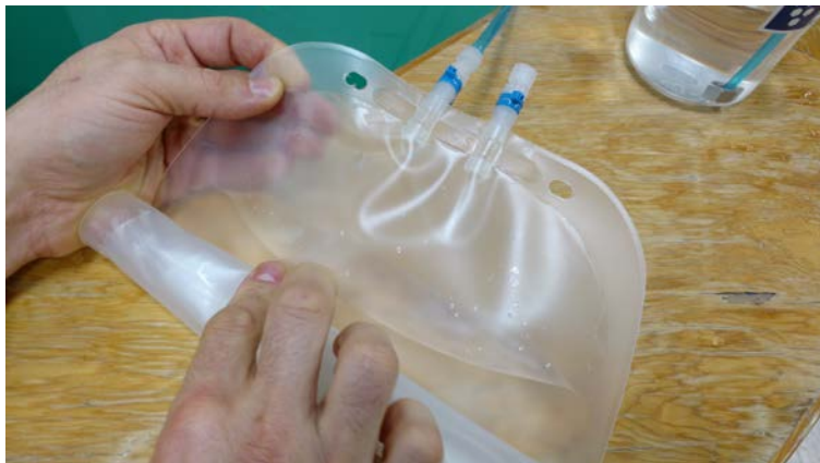
Figure 6-10: Roll Fixative Bag to Release Air
