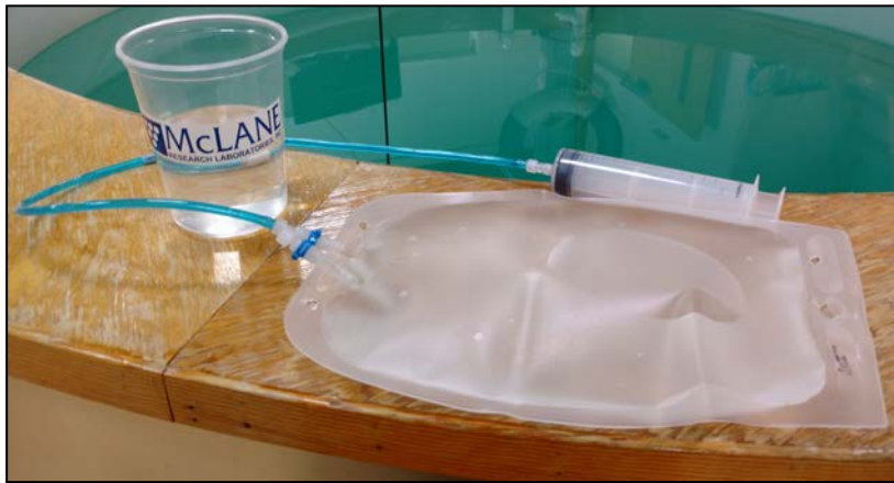
Figure 6-7: Inject Syringe Contents into Fixative Bag
