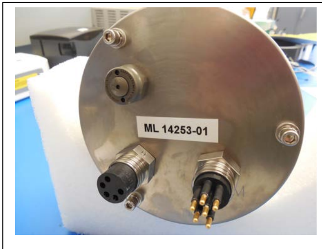
Figure 4-2: Releasing Pressure Relief Valve (Flat Style)
