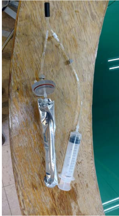
Figure 6-13: Fill Antifouling Tube
