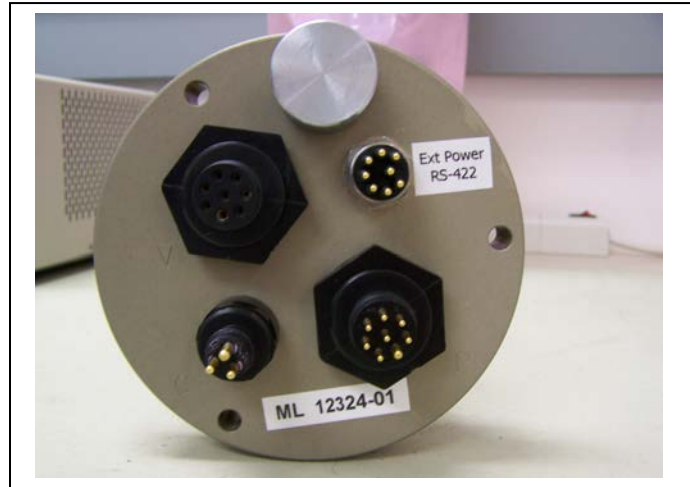
Figure B-1: Endcap with External Power and RS-422 Option
