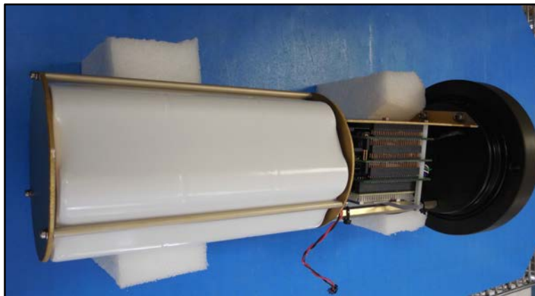
Figure 2-13: A21-1000 Battery Pack
