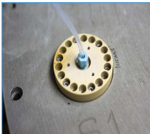
Figure 1-14: Sampling tube connected to Intake Port
