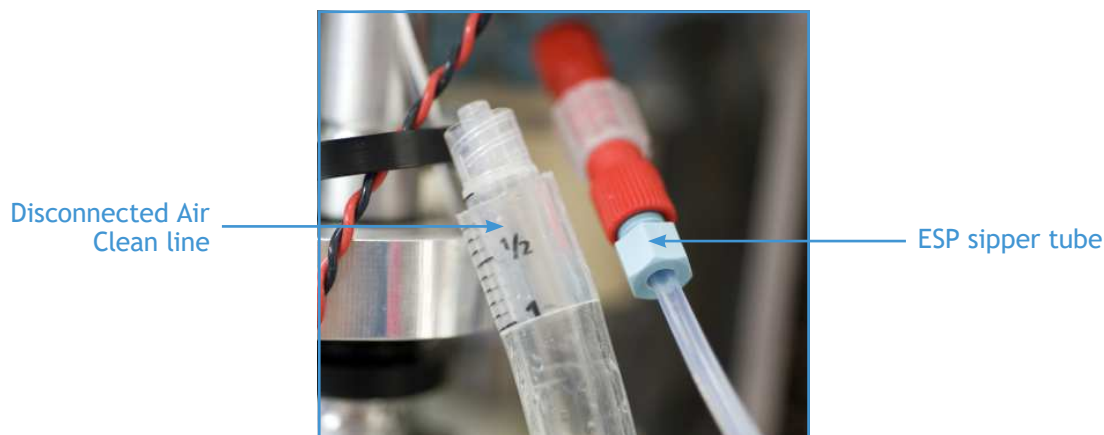
Figure 1-12: ESP sipper tube connected to Air Clean line
