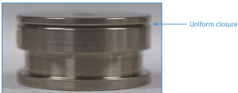
Figure 1-14: Uniform closure in properly assembled puck
