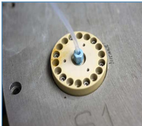
Figure 1-9: Supply line connected to Intake Port
