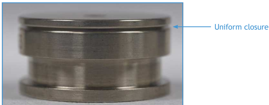
Figure 1-16: Uniform closure in properly assembled puck
