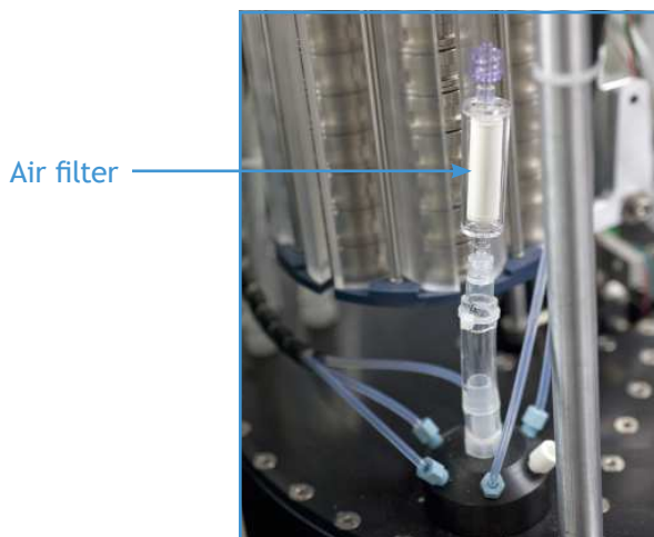
Figure 1-12: Air filter attached to exhaust tube
