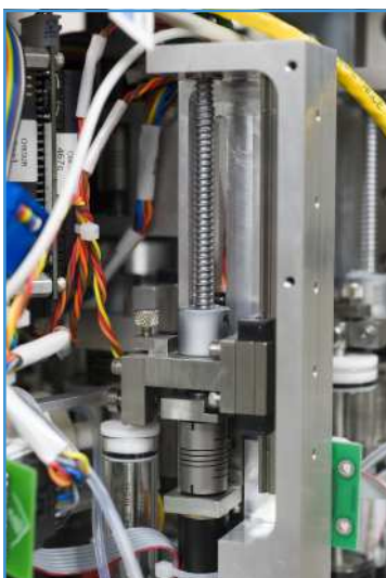
Figure 1-6: Syringe ballscrew assembly
