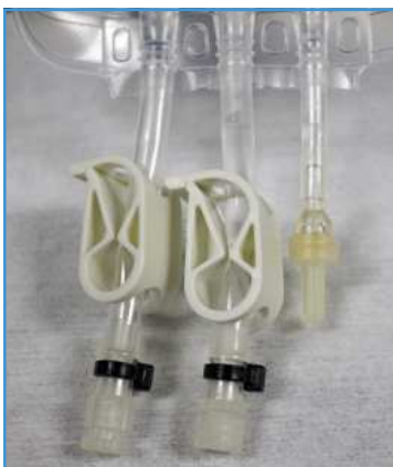
Figure 1-15: Male and female connectors on reagent bag
