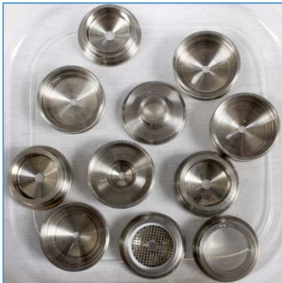
Figure 1-10: Pucks arranged for cleaning
