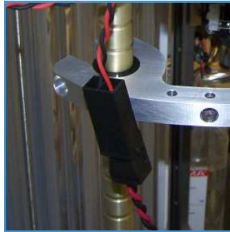
Figure 1-6: Power cable connected to ESP
