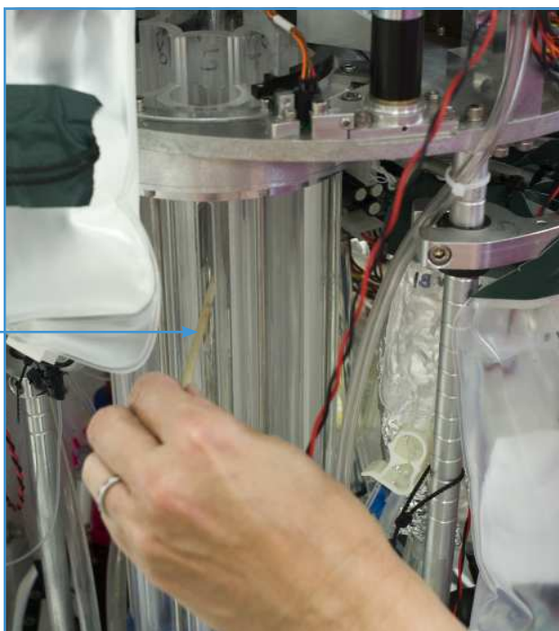
Figure 1-18: Support for loading pucks
