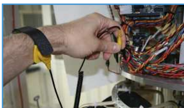
Figure 1-1: ESD wrist strap with attachment clip
