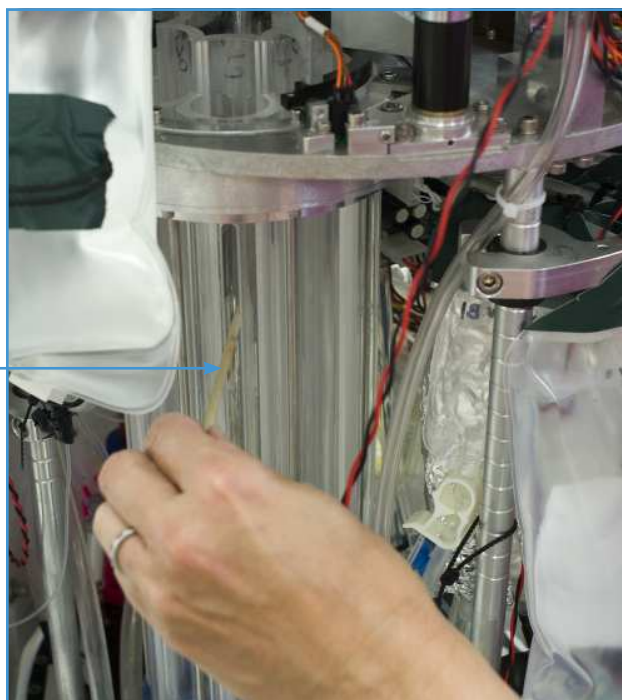
Figure 1-10: Support for loading pucks
