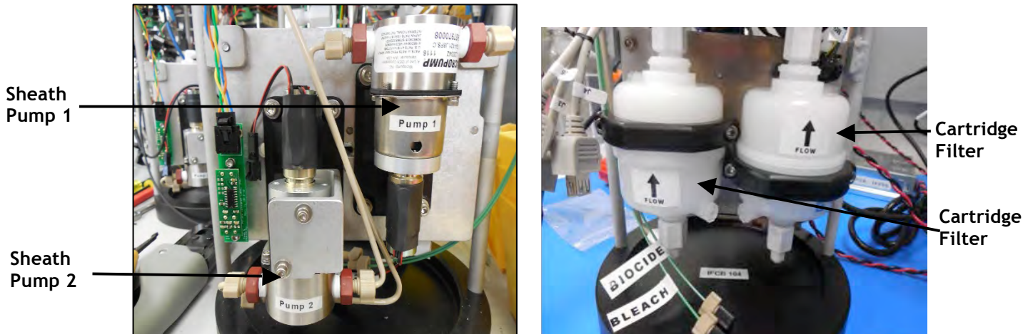
Figure 4-5: Sheath Pump 1 and 2
