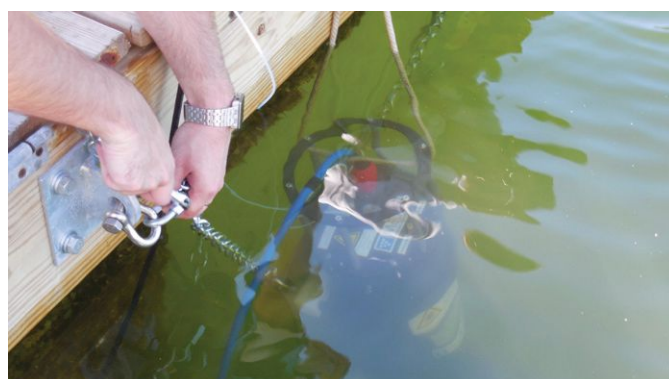
The Imaging FlowCytobot (IFCB) is an in-situ automated submersible imaging flow cytometer that generates images of particles in-flow taken from the aquatic environment.
