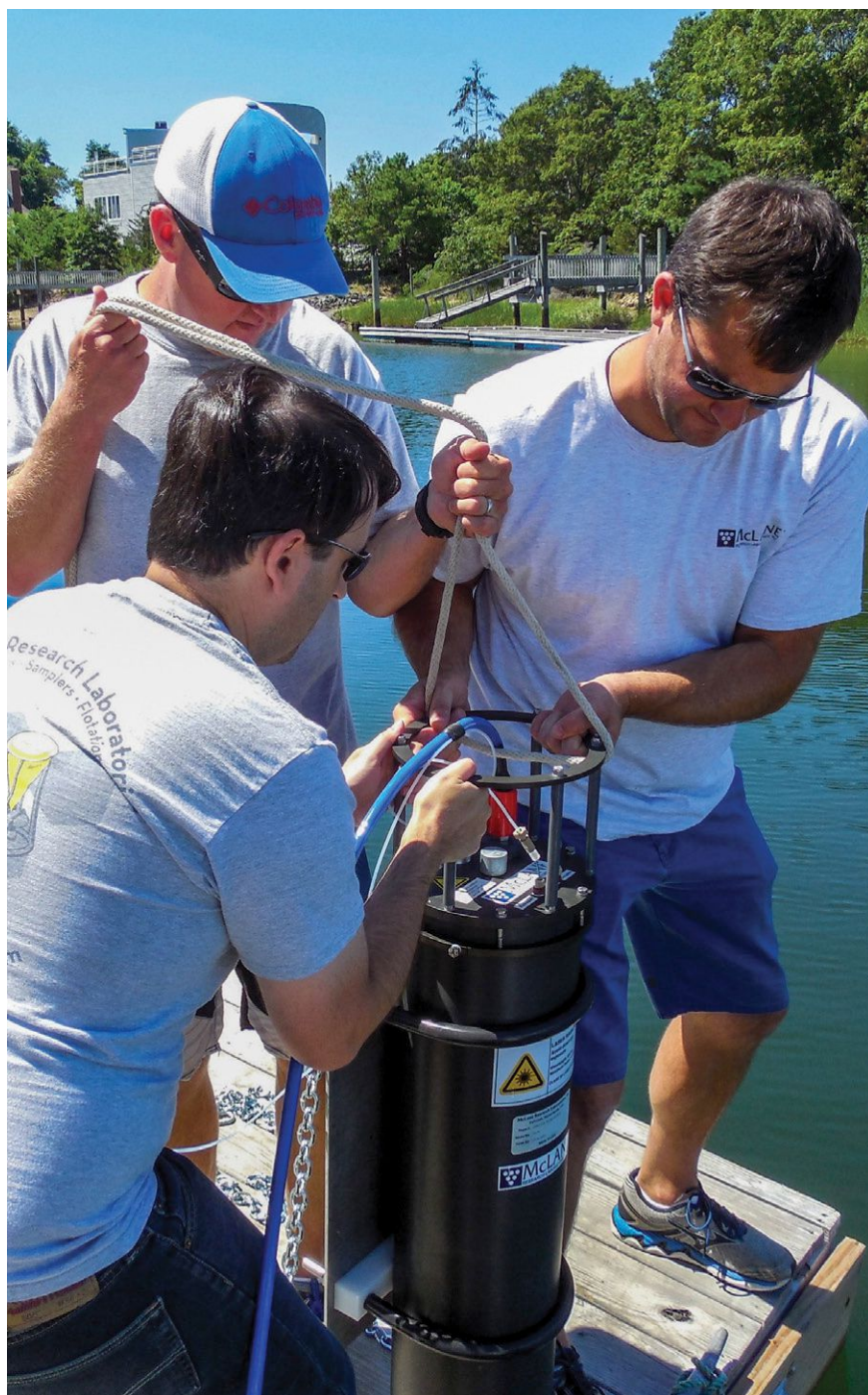
The IFCB is a fully submersible instrument with self-cleaning protocols to combat biofouling.
