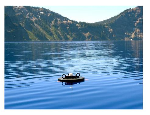
measurements, and the SUNA is a nitrate sensor. The FLBB(RT)/D is a combined fluorometer and turbidity sensor.
