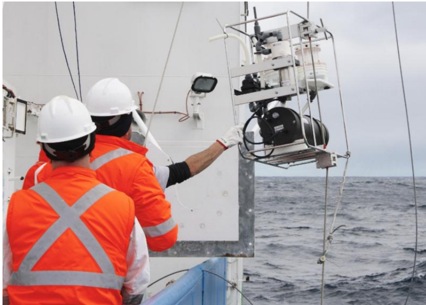
Dual Filter WTS-LV Deployment (Photo: Dr. K. Wuttig)
