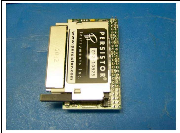
*Figure H-5: CF2 Micro Controller Board*
