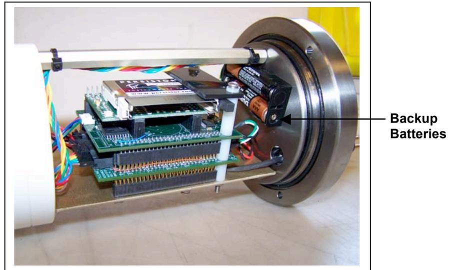
*Figure H-9: Sediment Trap Backup Batteries*
