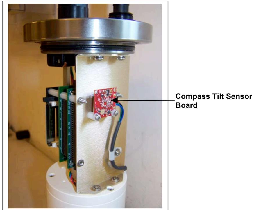
*Figure H-7: Compass Tilt Sensor Board*
