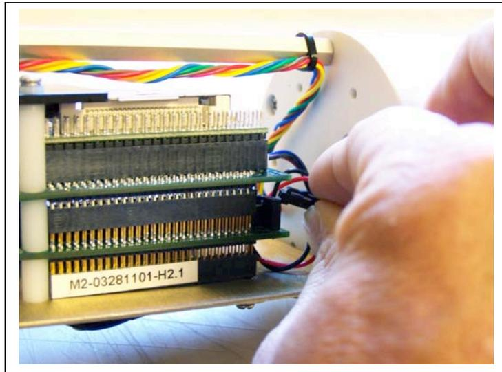
*Figure H-10: Connecting the Battery*
