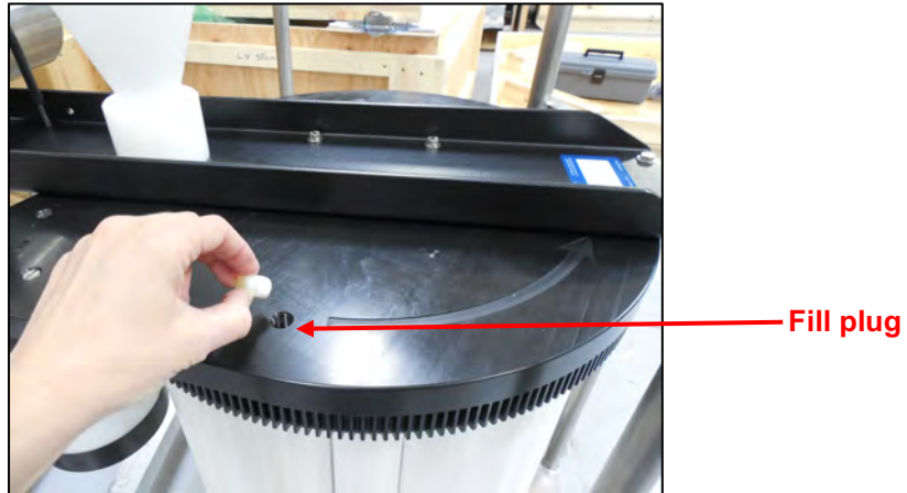
Figure 4.4-1: Removing the Plug from the Fill Hole
