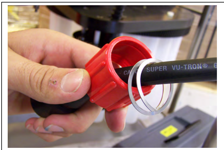
Figure E-4: Slide Locking Collar Off Motor Cable and Twist Off Locking Ring
