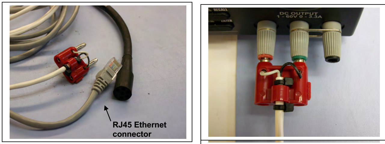
Figure D-2: Test Cable Connectors
