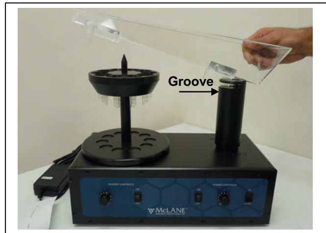
Figure A-3: Installing Sample Tray into Groove
