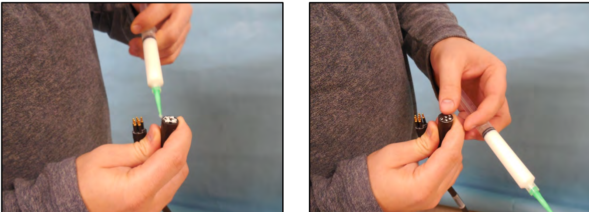
Figure B-7: Apply Molykote to RBR cable
