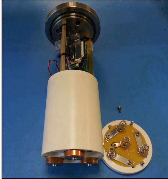
Figure 6.2-9: Controller End Cap Attached to Battery Holder
