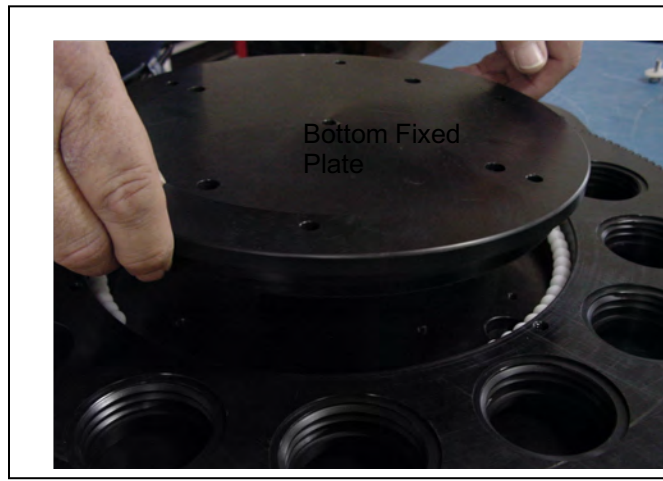
Figure 6.2-20: Removing Bottom Fixed Plate
