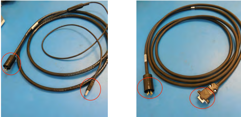
Figure 1-17: Gen3 Com Cable (USB Connector), and CF2 Com Cable (DB9 Serial Connector)
