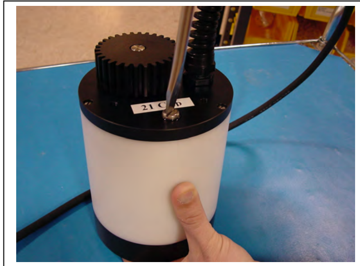
Figure 6.2-4: Back Off Fill Hole Screw and Press Up on Bladder
