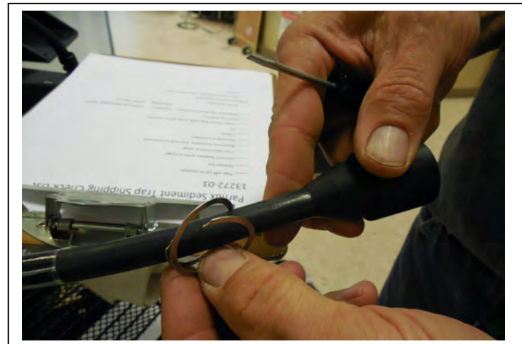
Figure E-4: Slide Locking Collar Off Motor Cable and Twist Off Locking Ring
