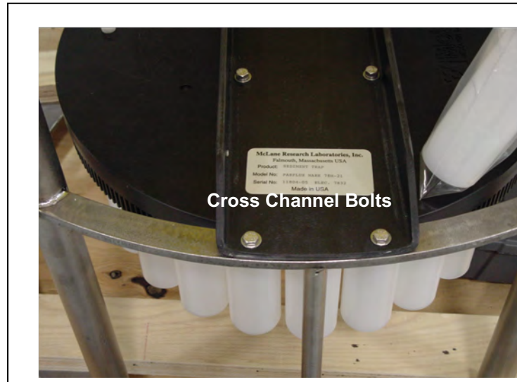
Figure 6.2-16: Remove Cross Channel From Frame
