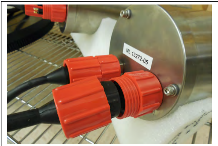
Figure E-2: Unscrew Locking Collar and Unplug Bulkhead Connector
