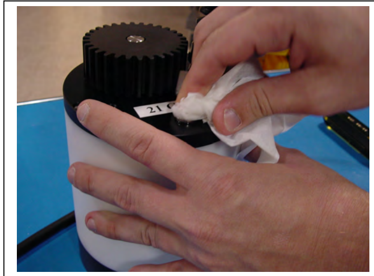
Figure 6.2-6: Cleaning Excess Oil from Fill Plug
