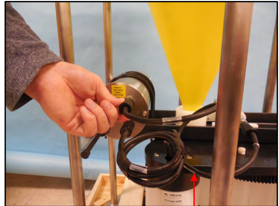
Cable on the inside of frame
