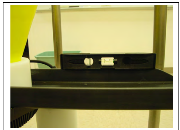
Figure 4.5-4: Confirm that the Sediment Trap is Level
