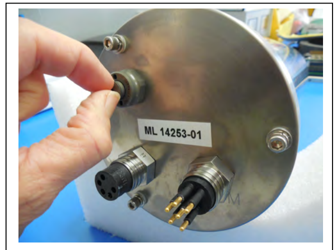
Figure 2-2: Releasing Pressure Relief Valve (Flat Style)
