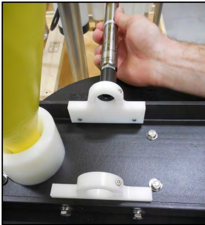
Figure B-3: Slide RBR sensor into mounting brackets. Do not slide past the red label.
