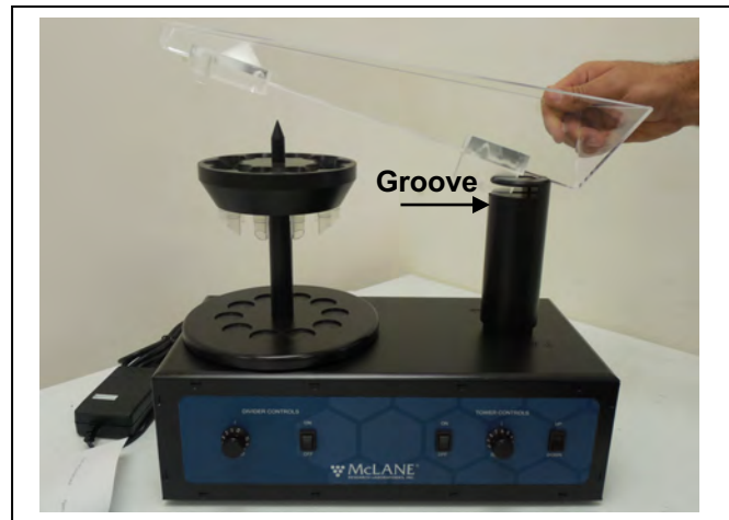
Figure A-3: Installing Sample Tray into Groove
