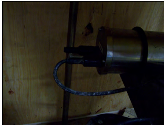
Figure 6.1-1: Results of Poor Rinsing After Deployment
