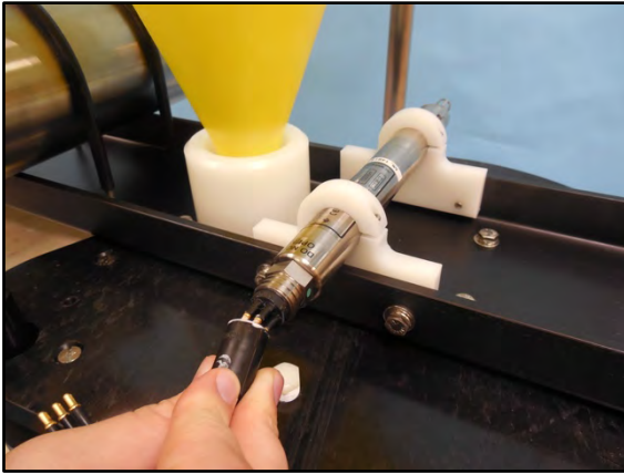
Figure B-8: Connect RBR sensor cable to sensor and tighten locking sleeve
