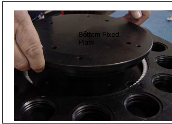
Figure 6.2-20: Removing Bottom Fixed Plate
