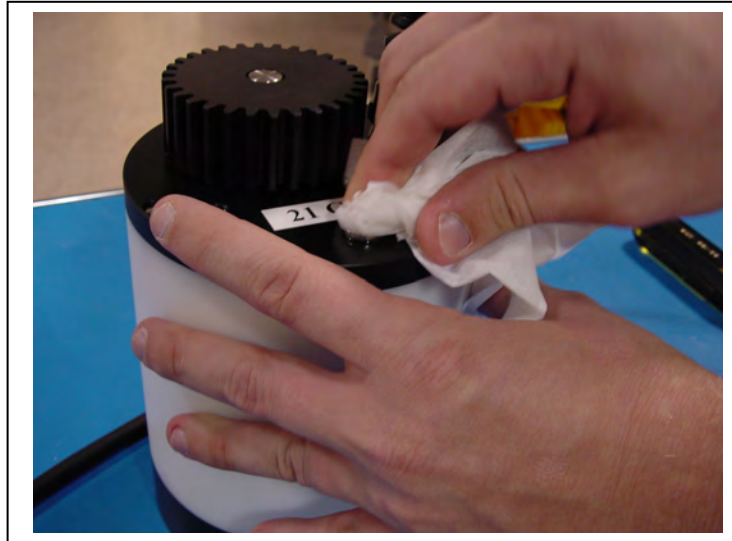
Figure 6.2-6: Cleaning Excess Oil from Fill Plug
