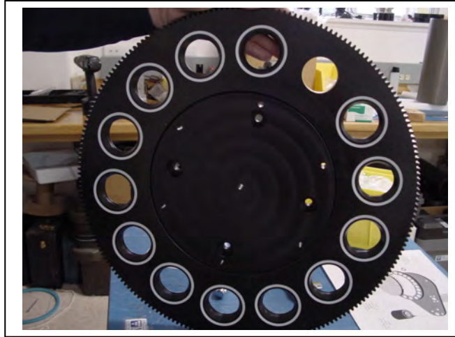
Figure 6.2-18: Variseals® in Gear Ring Grooves
