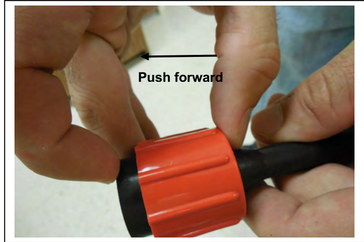
Figure E-8: Push Red Collar Towards Bulkhead
