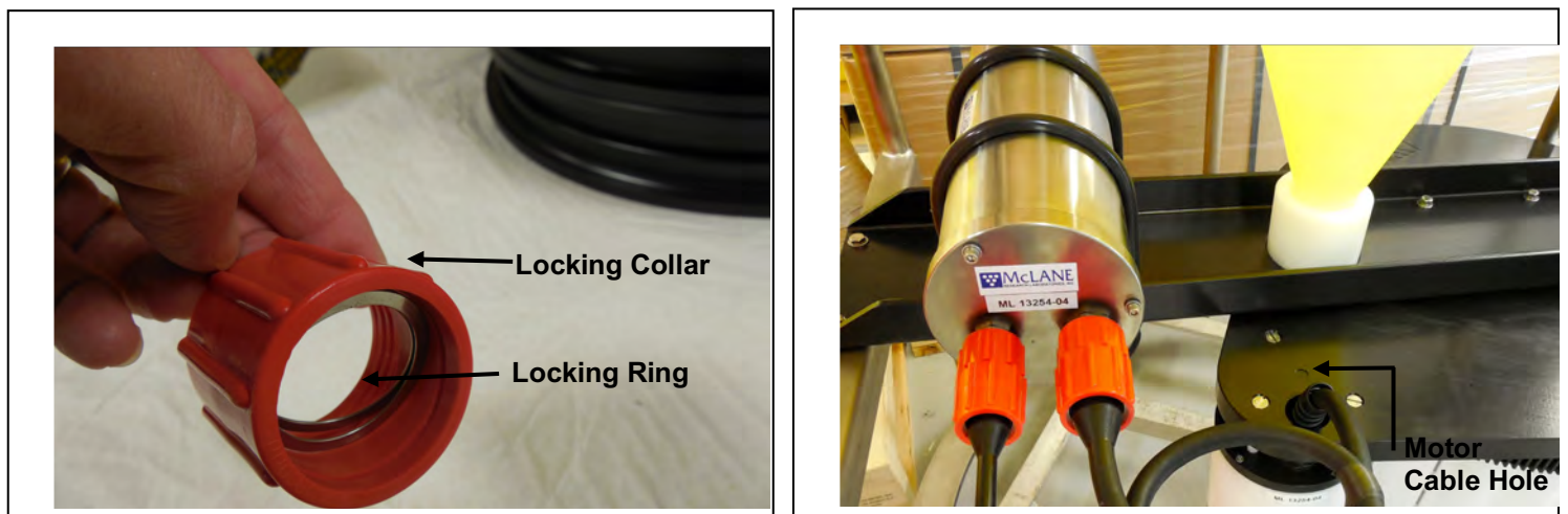
Figure E-1: High Pressure Penetrators with Locking Collar and Inner Locking Ring
