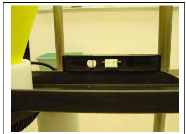
Figure 4.5-4: Confirm that the Sediment Trap is Level
