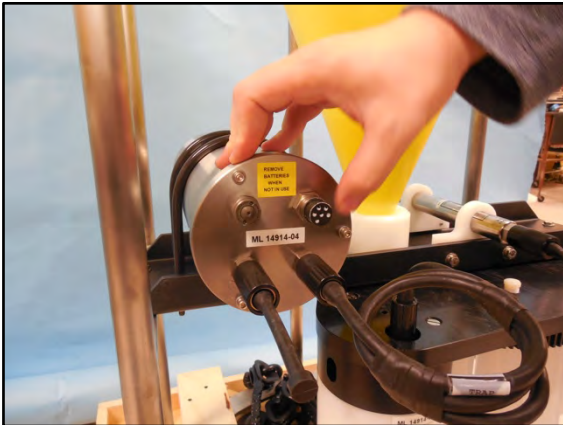
Figure B-9: Connect RBR sensor cable to controller housing
