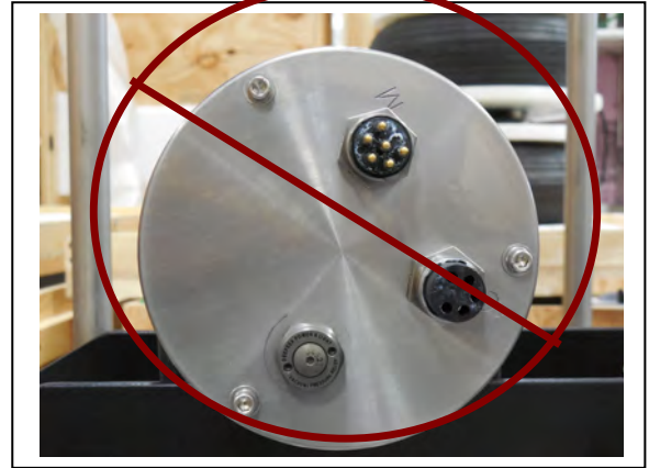
Figure 4.5-3: Incorrect Controller Housing Orientation with Tilt Sensor
