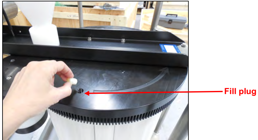
Figure 4.4-1: Removing the Plug from the Fill Hole
