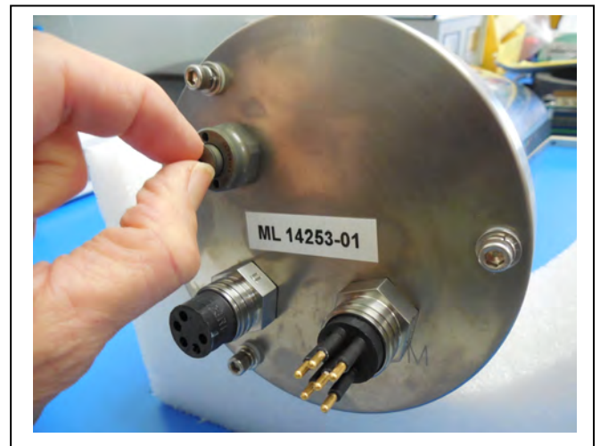
Figure 2-4: Releasing Pressure Relief Valve (Flat Style)
