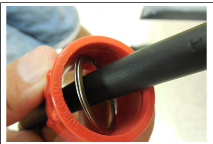
Figure E-7: Fit Silver Locking Ring Inside Locking Collar Groove
