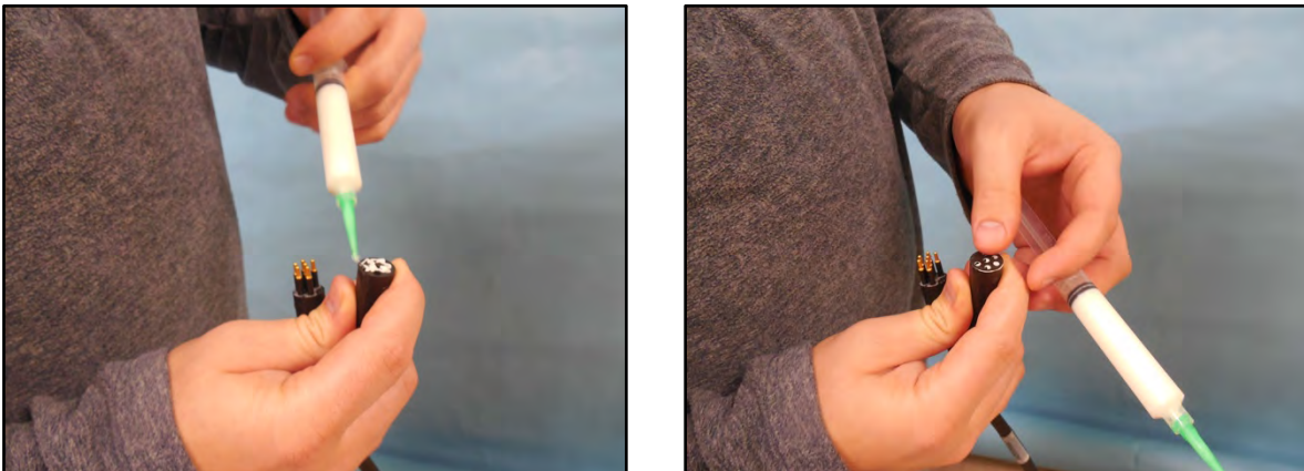
Figure B-7: Apply Molykote to RBR cable
