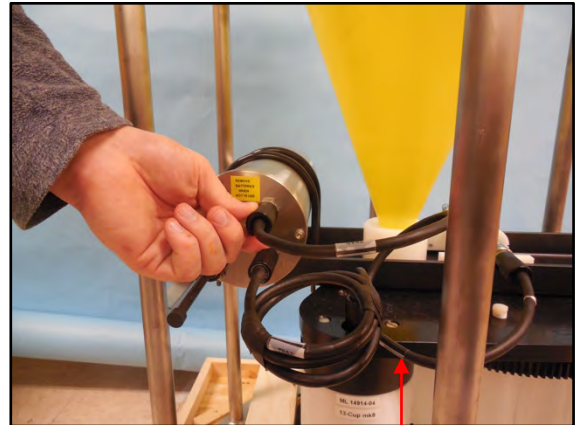
Figure B-9: Connect RBR sensor cable to controller housing
