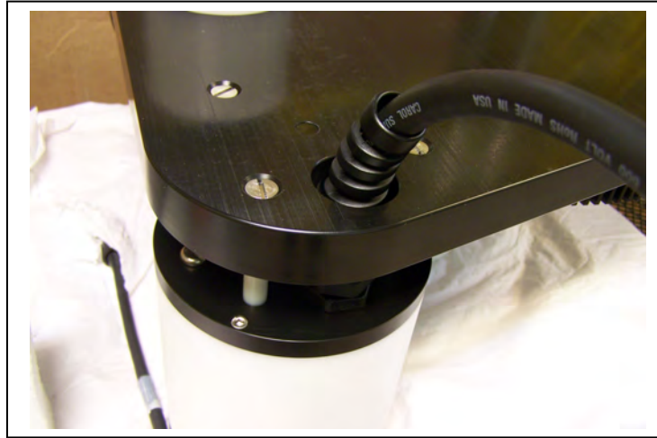
Figure E-5: Fit Motor Cable Down Through Hole in Rotator Plate
