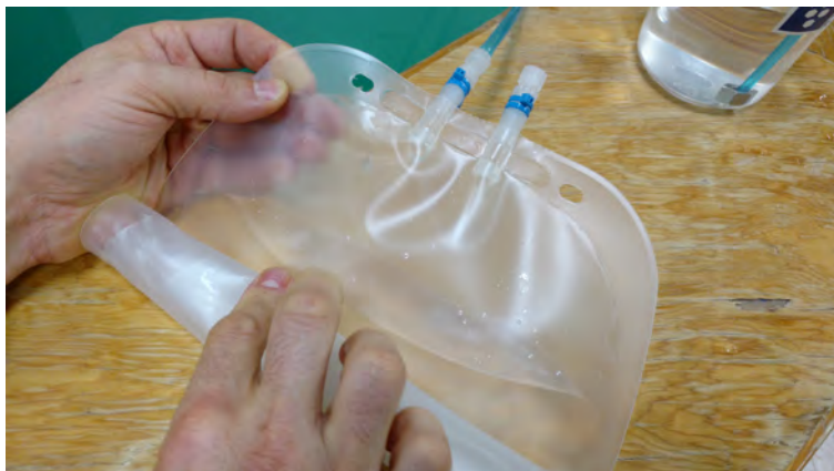
Figure 6-10: Roll Fixative Bag to Release Air
