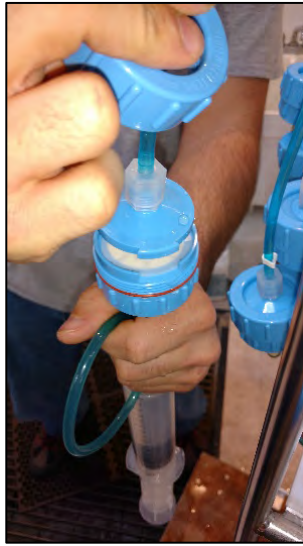
Figure 6-4: Reattaching Top and Bottom of Filter
