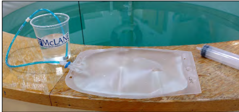
Figure 6-8: Place Hose-F into Fixative Container
