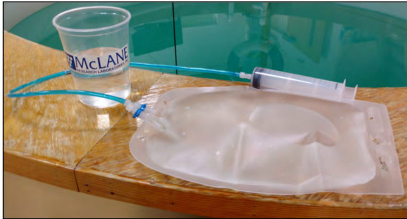
Figure 6-7: Inject Syringe Contents into Fixative Bag
