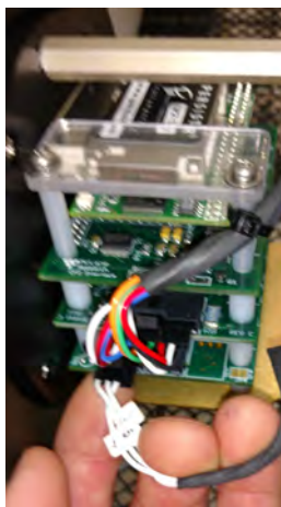
Figure E-4: Plug MTE Connector into Loopback Tester
