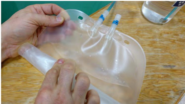
*Figure 4.2-5: Roll Fixative Bag to Release Air*
