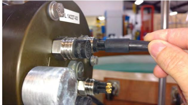
*Figure 2.3-5: Connecting the COM Cable*
