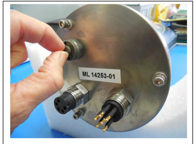
*Figure 2.3-1: Releasing Pressure Relief Valve (Flat Style)*
