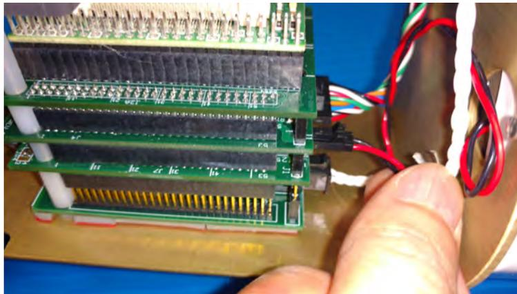
*Figure 2.3-4: Connecting the Battery*
