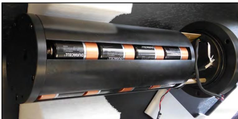
*Figure 1-16: Drop-in Battery Holder for 'D' Cell Batteries*
