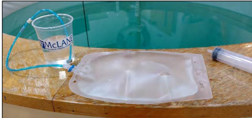
*Figure 4.2-3: Place Hose-F into Fixative Container*
