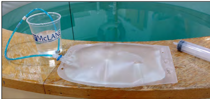
Figure 4.3-6: Place Hose-F into Fixative Container
