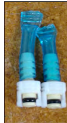
Figure 4.3-7: Pinch Fixative Bag Hose, Attach to Intake-2 Hose
