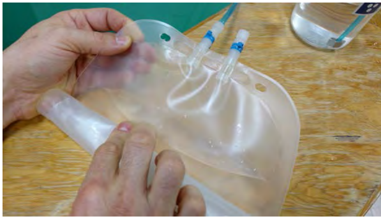
Figure 4.3-8: Roll Fixative Bag to Release Air
