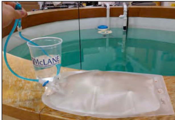
Figure 4.3-7: Pinch Fixative Bag Hose, Attach to Intake-2 Hose
