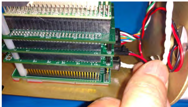
Figure 2.3-4: Connecting the Battery
