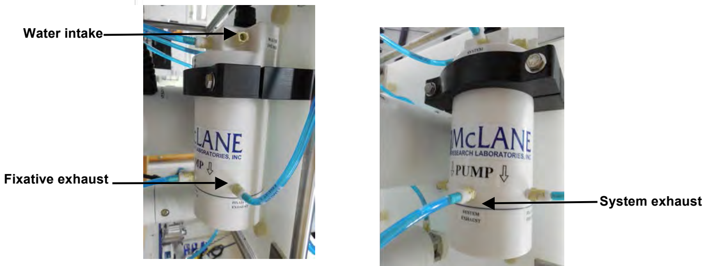
Figure 1-11: Fixative Valve Water Intake, Fixative and System Exhausts
