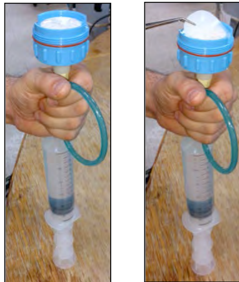
Figure 4.1-3: Injecting Water with Syringe
