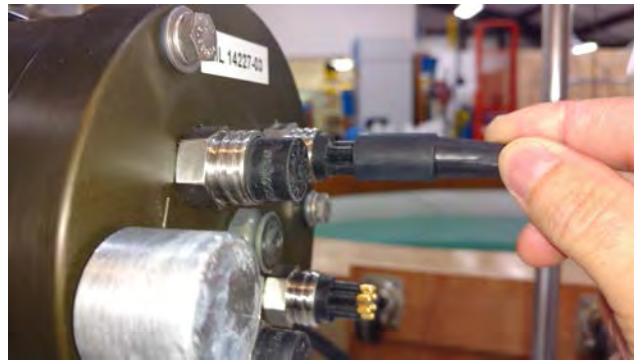
Figure 2.3-5: Connecting the COM Cable
