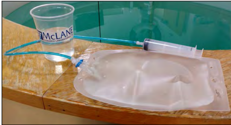
Figure 4.3-5: Inject Syringe Contents into Fixative Bag
