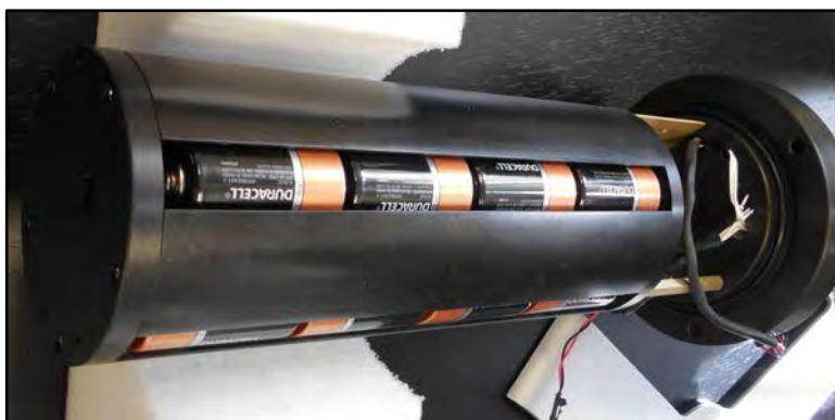
Figure 1-16: Drop-in Battery Holder for 'D' Cell Batteries
