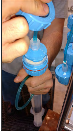
Figure 4.1-4: Reattaching Top and Bottom of Filter
