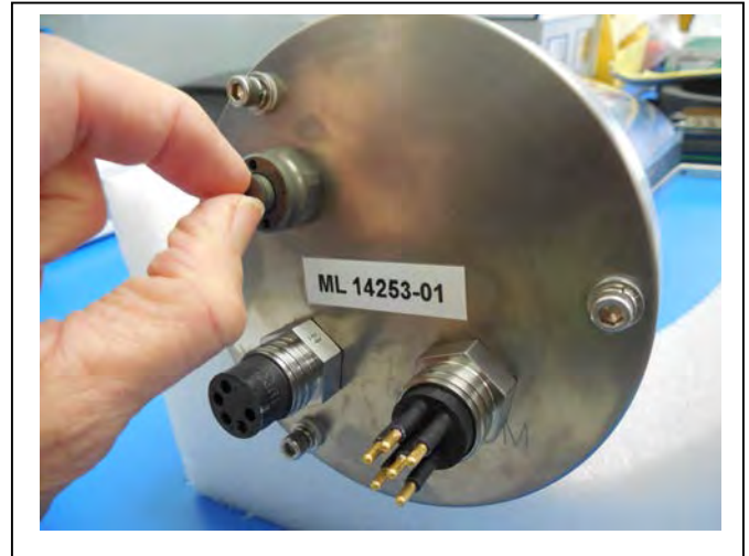
Figure 2.3-1: Releasing Pressure Relief Valve (Flat Style)
