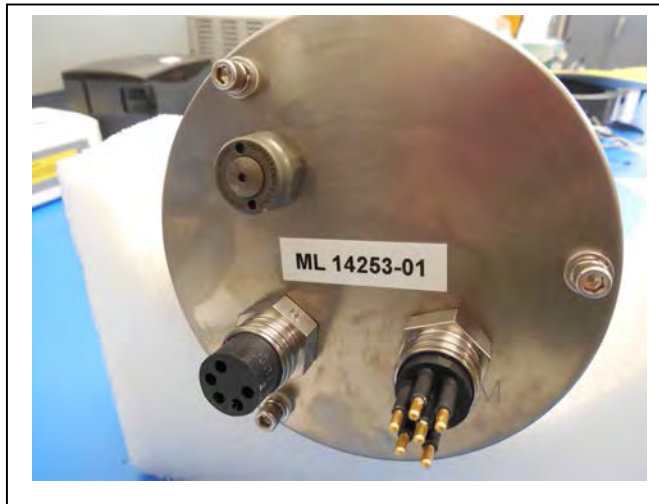
Figure 2.3-1: Releasing Pressure Relief Valve (Flat Style)
