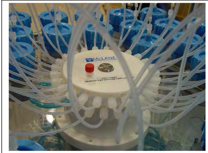
*Figure 6-4: Intake Cap*
