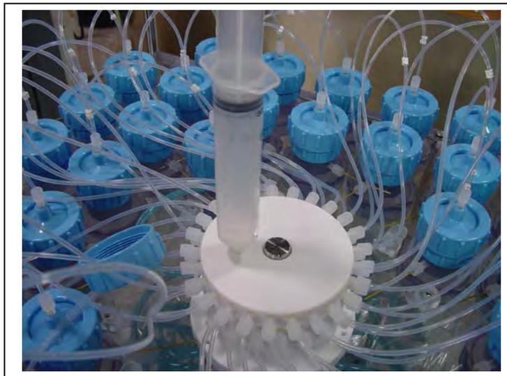
*Figure 6-12: Injecting Water into the Valve Intake*
