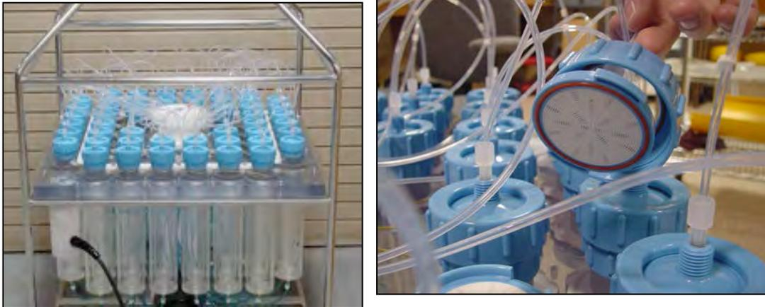
*Figure 4-8: RAS-500 with Optional Filter Holder on each Sample*
