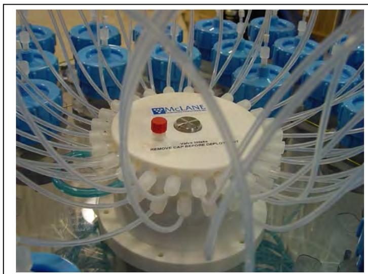
*Figure 3-22: Intake Cap*
