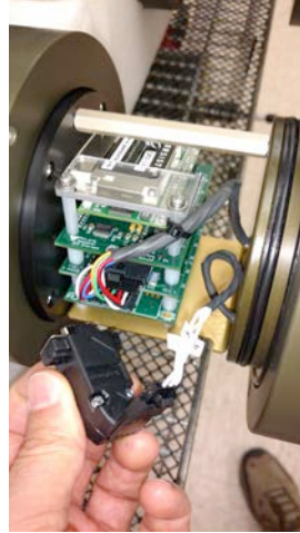
Figure 4: Plug MTE Connector into Loopback Tester
