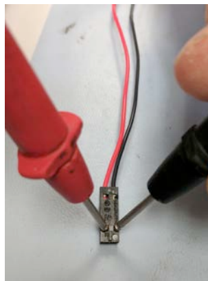
Figure 1: Measuring Battery Connector Voltage
