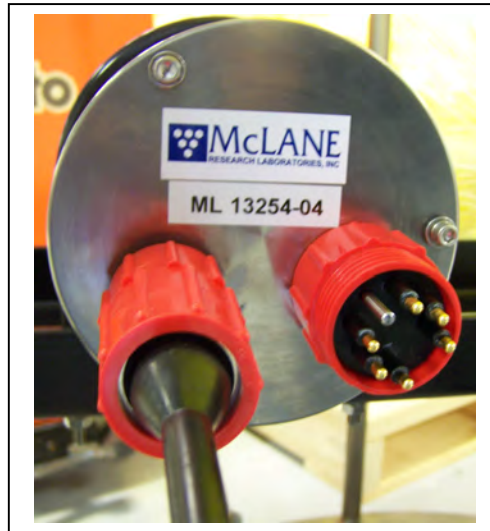
Figure 1-9: Deep Controller Housing End Cap Bulkhead Connectors
