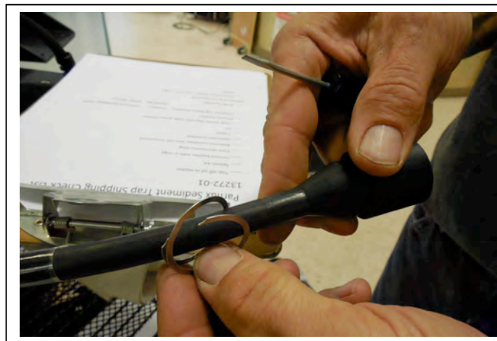
Figure E-4: Slide Locking Collar Off Motor Cable and Twist Off Locking Ring
