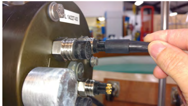
Figure 2.3-5: Connecting the COM Cable
