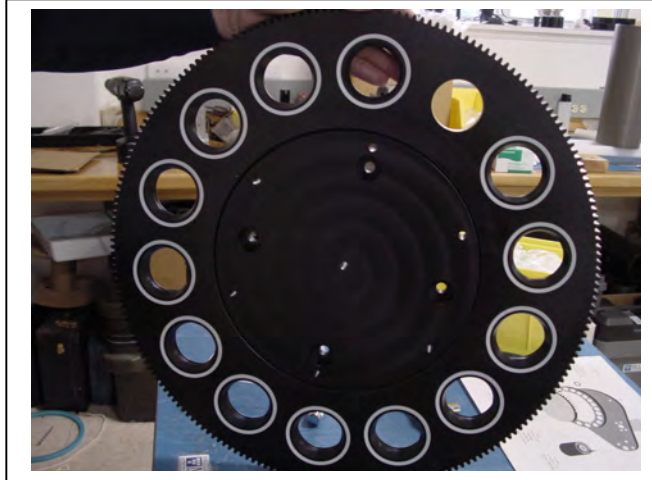
Figure 6.2-18: Variseals® in Gear Ring Grooves
