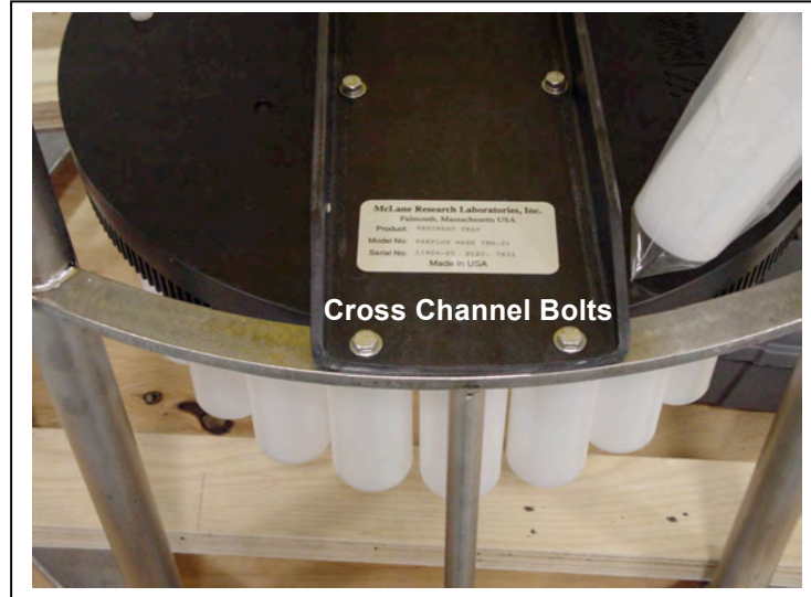
Figure 6.2-16: Remove Cross Channel From Frame
