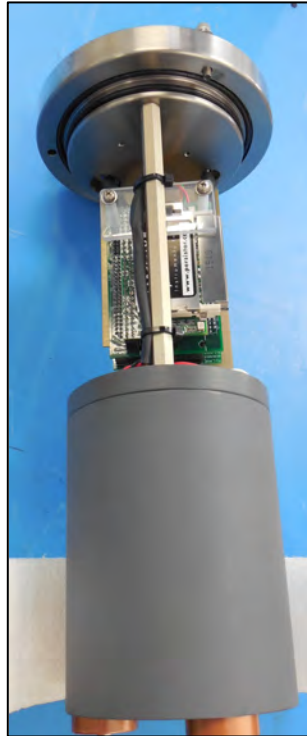
Figure 6.2-9: Controller End Cap Attached to Battery Holder
