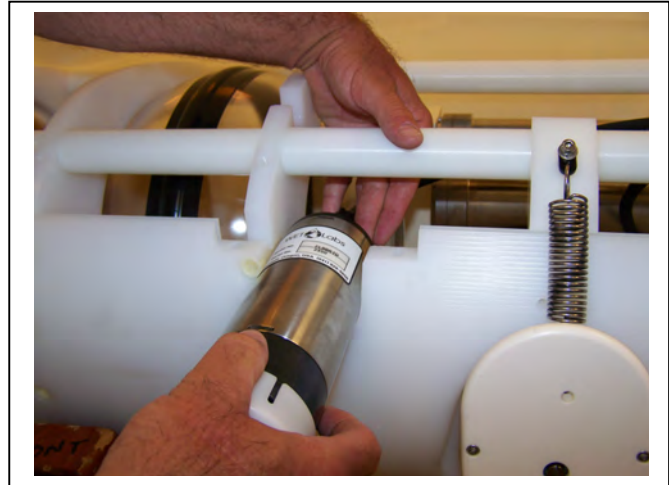
Figure 6.2-6: Placing the Sensor in the Mount
