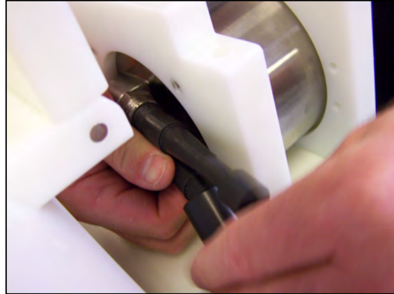
Figure 3.1-23: Detach Bulkhead Connector
