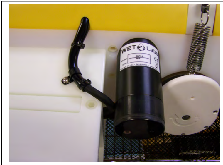
Figure 6-11: BBFL2 Model- Installed
