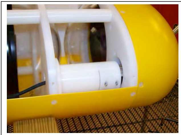
Figure 9-15: Pulling Out the Sensor Clamp
