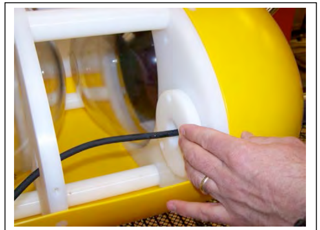
Figure 9-10: Re-inserting the Clamp
