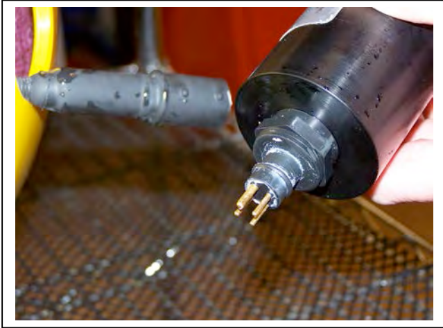
Figure 9-7: Connecting to the Bulkhead
