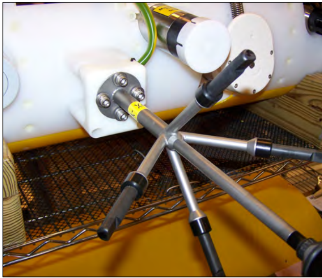
Figure 4-1: MMP with FSI ACMPlus
