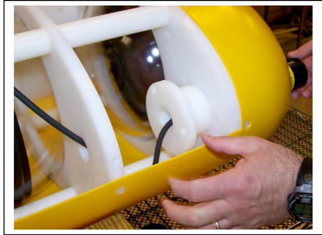
Figure 9-14: Loosening the Sensor Clamp
