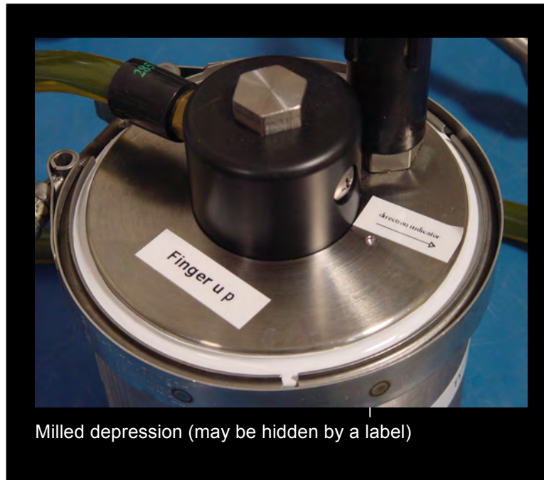
Figure 4-19: Correct Positioning of ACMPlus Electronics Housing
