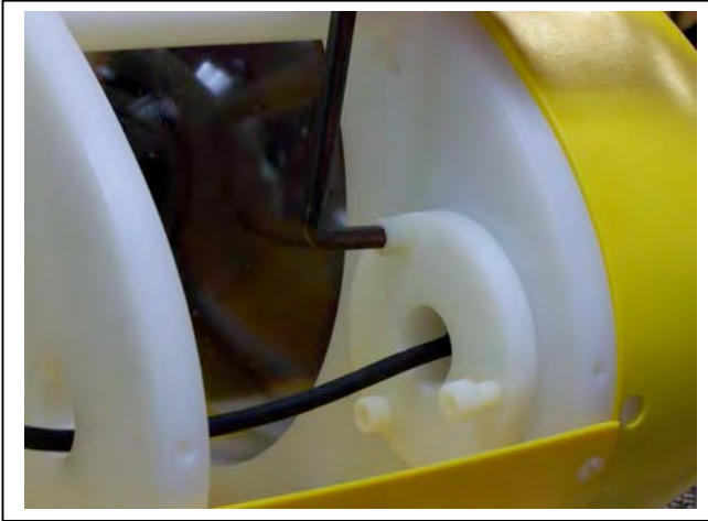
Figure 9-11: Tightening the Socket Cap Screws
