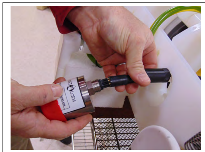
Figure 6.4-11: Remove the Sensor Cable
