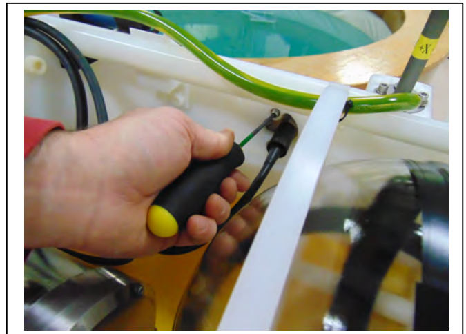
Figure 6.4-10: Loosen Mounting Screws
