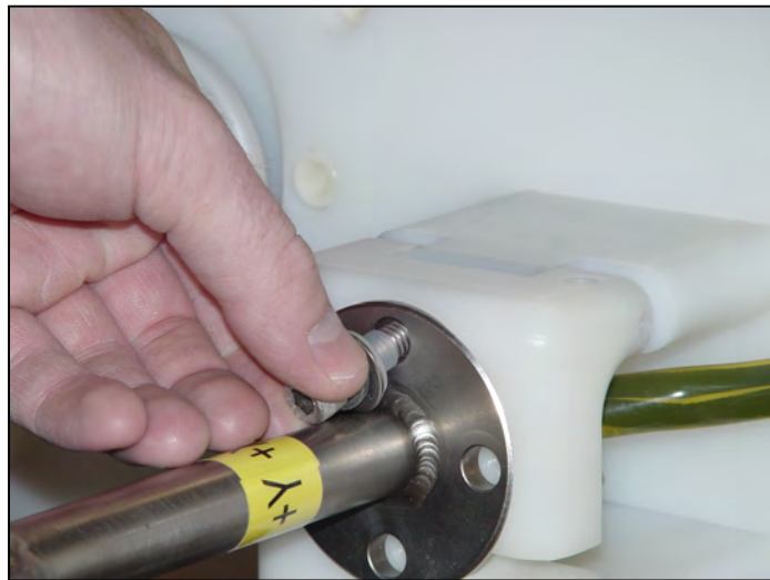
Figure 4-16: Tighten ACM+ Sting
