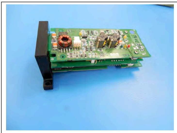
Figure B-1: Sea-Bird UIM Modem Electronics Board
