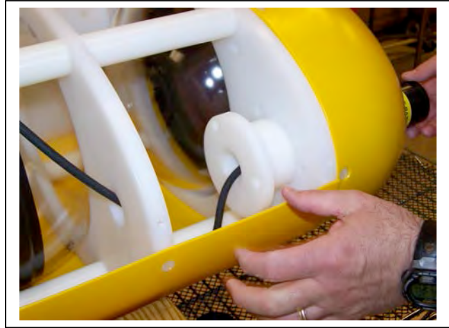
Figure 9-14: Loosening the Sensor Clamp
