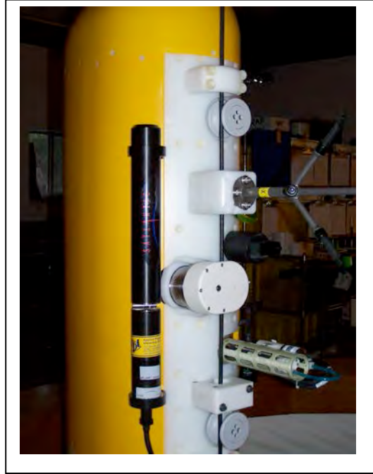
Figure 8-21: Completed SUNA Installation
