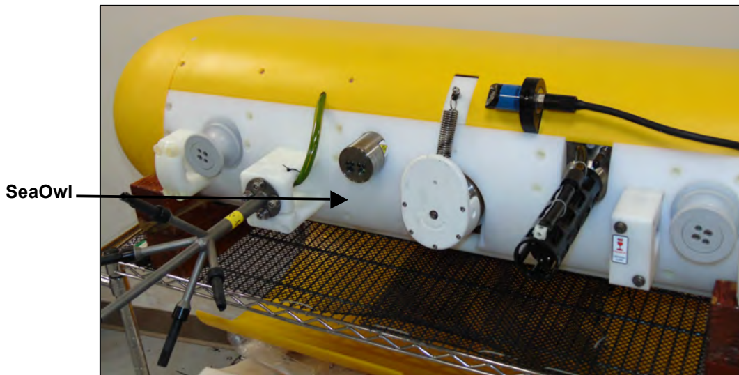
Figure 6.4-1: MMP with SeaOwl Installed
