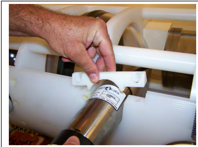
Figure 6.2-7: Placing the Mounting Support
