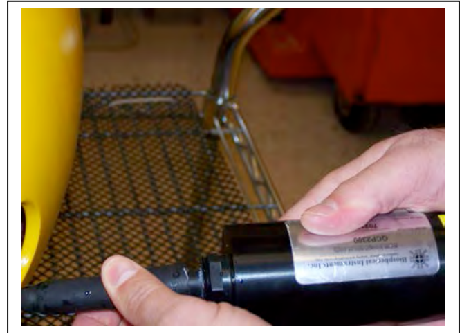
Figure 9-18: Removing Bulkhead Connector
