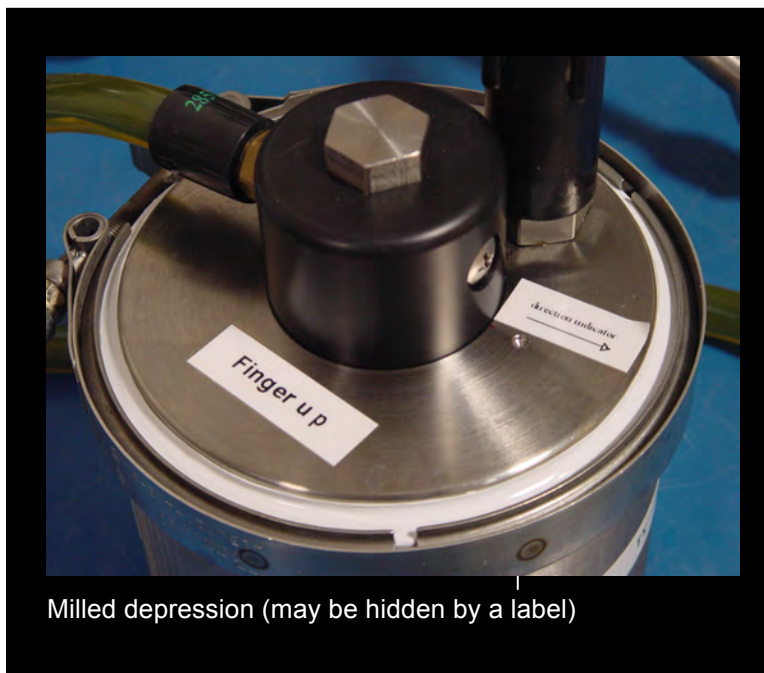
Figure 4-19: Correct Positioning of ACM+ Electronics Housing
