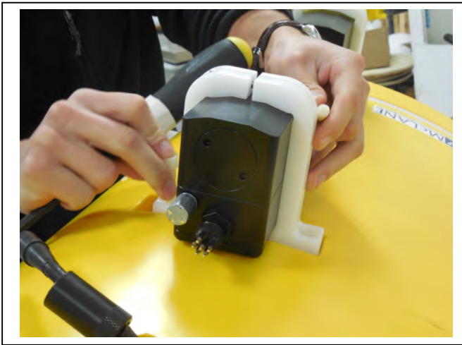
Figure 6.3-13: Securing Top Clamp
