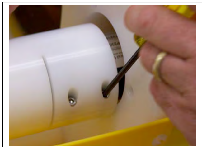
Figure 9-16: Loosening the Clamp Screws
