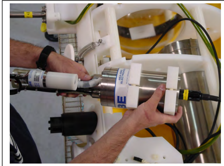
Figure 1.1-11: Lifting the CTD from the Sensor Mount
