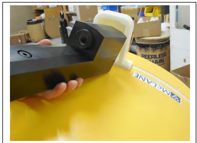
Figure 6.3-12: Inserting the C-Star
