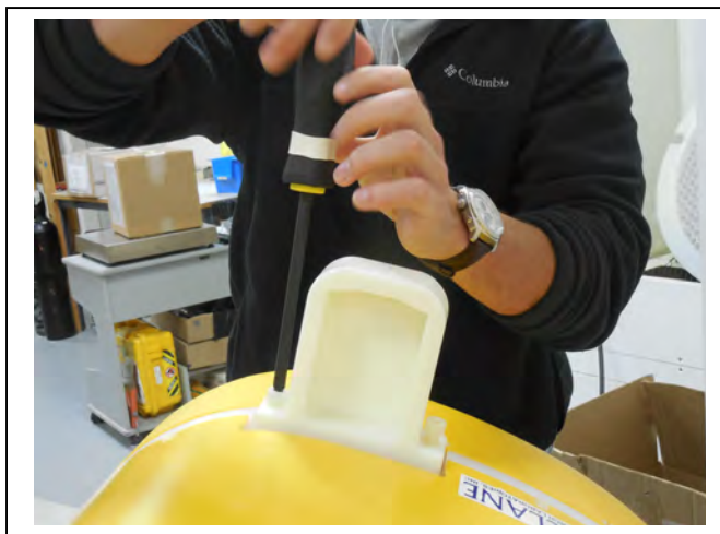
Figure 6.3-11: Tightening Nylon Screws
