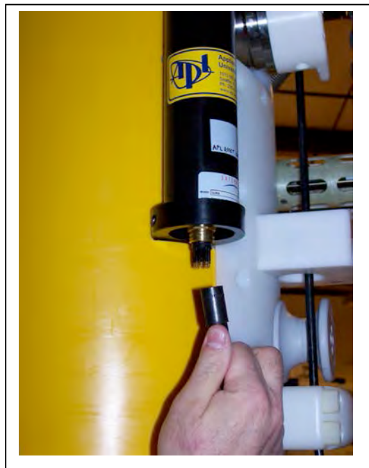
Figure 8-19 and Figure 8-20: Connect the 5-pin connector
