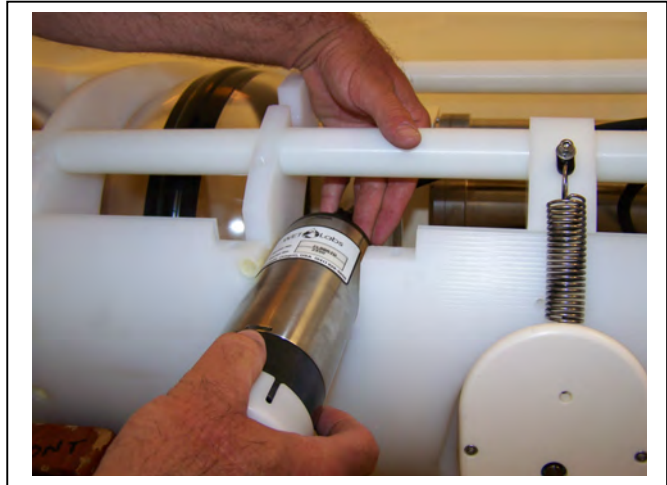
Figure 6.2-6: Placing the Sensor in the Mount
