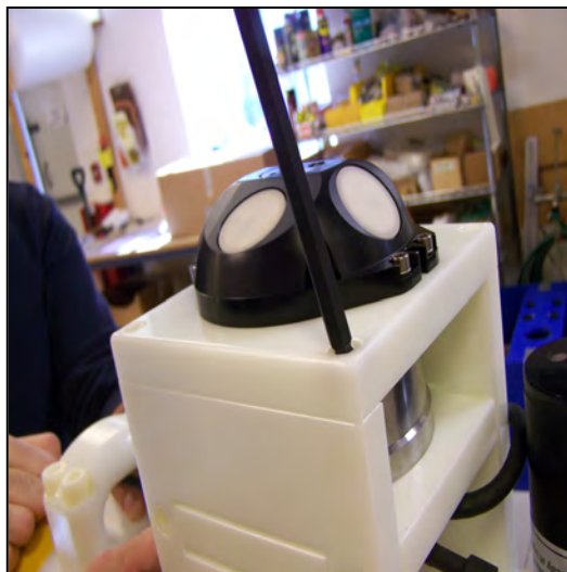
Figure 3.1.28: Tighten Hinge Plate Screws
