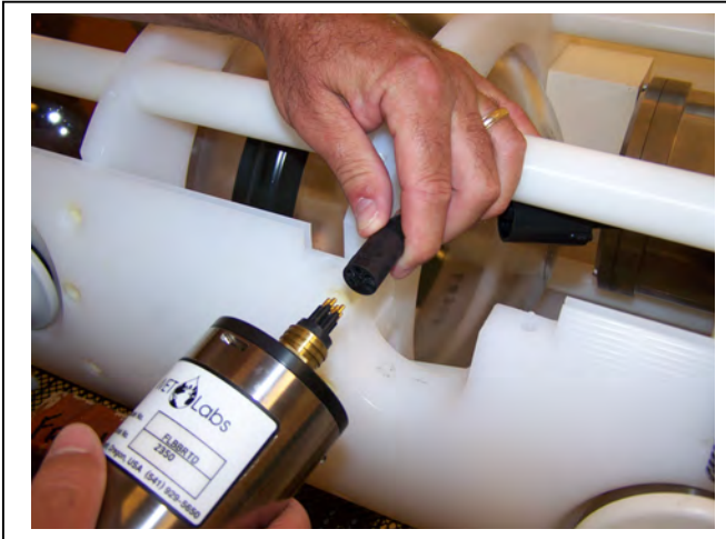
Figure 6.2-5: Connecting the Sensor Cable
