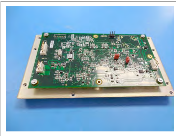
Figure 11.2-1: MLM Modem Electronics Board and Inductive Coil
