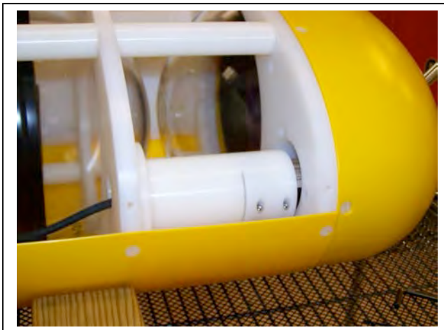
Figure 9-15: Pulling Out the Sensor Clamp
