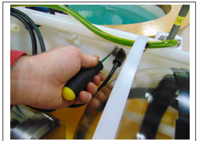
Figure 6.4-10: Loosen Mounting Screws
